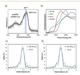
Fig. 3 (a) XPS profiles for the Mn  $2p_{3/2}$  region for Mn NPs and (b) Mn K-edge XANES spectra of the reference Mn compounds and Mn NPs, and (c) Fourier-transformed  $k^3$ -weighted Mn K-edge EXAFS spectra of Mn NPs\_before reaction (Mn NPs\_br) and (d) after reaction (Mn NPs\_ar).
