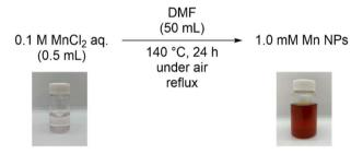
Scheme 2 Synthesis of DMF-stabilized manganese nanoparticles.
