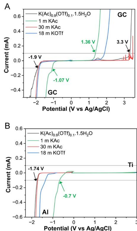
Fig. 4 Linear sweep voltammetry (LSV) profiles recorded at a scan rate of  $1 \text{ mV s}^{-1}$  for the solutions  $\text{K}(\text{Ac})_{0.9}(\text{OTf})_{0.1} \cdot 1.5\text{H}_2\text{O}$ , 1 m KAc, 30 m KAc, and 18 m KOTf using a glassy carbon, GC, electrode (A) and Ti and Al foils (B) as working electrodes. The dotted lines indicate the potentials at which hydrogen and oxygen evolution reactions start occurring, defining the potential window.
