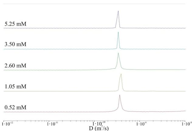
Fig. 6 Protection of distribution of diffusion coefficient derived from 2D DOSY spectra for various peptide concentrations: 0.52 mM (red), 1.05 mM (light green), 2.60 mM (green), 3.50 mM (blue), and 5.25 mM (purple).
