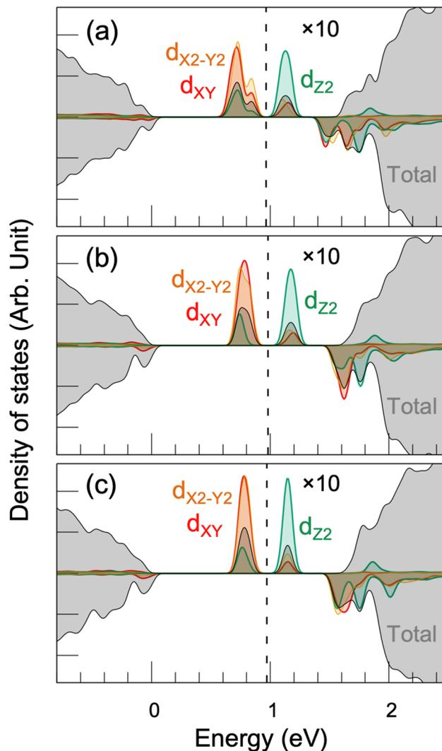
Fig. 5 Total and projected DOS for (a)  $2W_S$ - $2NN_{ZZ}$ , (b)  $2W_S$ - $3NN_{AC}$ , and (c)  $2W_S$ - $3NN_{ZZ}$  in  $WS_2$ . Black lines and gray shaded regions are the total DOS, and projected DOS are shown using the corresponding colors denoted in the figures. All the projected DOSs were scaled by a factor of 10 with respect to the total DOS. Valence band maximum was set to 0.0 eV, and the Fermi level is presented by the vertical dotted lines.
