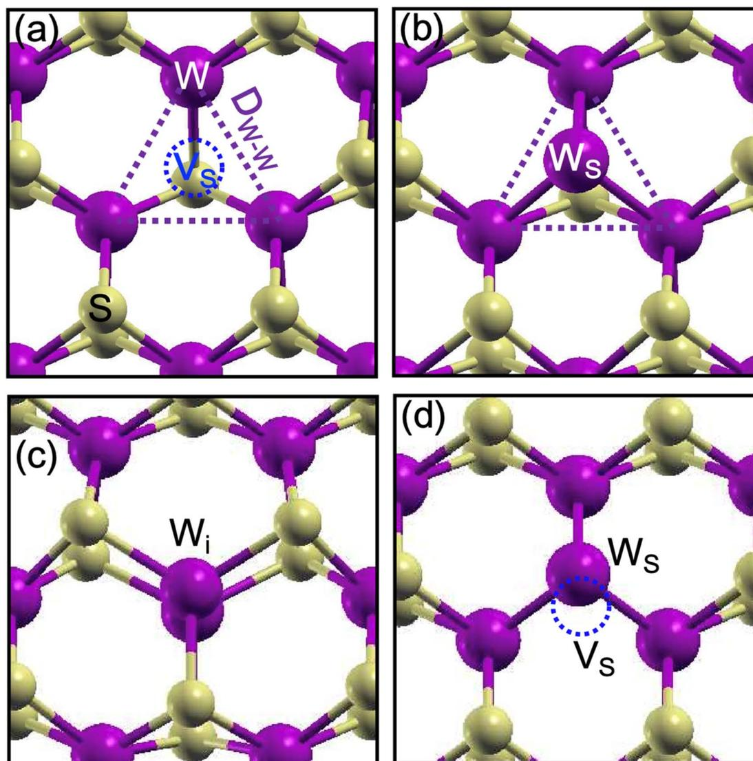
Fig. 1 Atomic structures of (a) S vacancy ( $V_S$ ), (b) W antisite ( $W_S$ ), (c) W interstitial ( $W_i$ ), and (d)  $W_S-V_S$  complex defects in  $WS_2$ . In (a) and (d), vacancy sites are denoted by dotted blue circles. In (a) and (b), the neighboring W atoms near the defect are denoted by dotted violet lines. The W and S atoms are represented by magenta and yellow balls, respectively.
