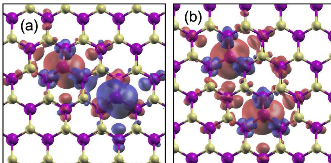
**Fig. 4** Spin density for (a) 2W<sub>S</sub>-2NN<sub>AC</sub> and (b) 2W<sub>S</sub>-2NN<sub>ZZ</sub> in WS<sub>2</sub>. Red (blue) contours represent the spatial distribution of the majority (minority) spin.
