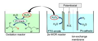
Fig. 1 The electrochemical setup for oxidative  $H_2O_2$  production from water with  $H_2$  evolution and the oxidation of allylic alcohol to  $\alpha,\beta$ -unsaturated aldehyde using the  $H_2O_2$  derived from 2e-WOR. R.E. is reference electrode.
