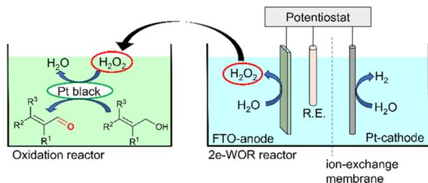
Fig. 1 The electrochemical setup for oxidative  $\text{H}_2\text{O}_2$  production from water with  $\text{H}_2$  evolution and the oxidation of allylic alcohol to  $\alpha,\beta$ -unsaturated aldehyde using the  $\text{H}_2\text{O}_2$  derived from 2e-WOR. R.E. is reference electrode.
