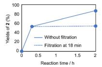
Fig. 2 Hot-filtration test in the H<sub>2</sub>O<sub>2</sub> oxidation of 1.
