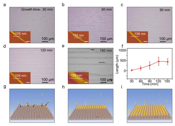
Fig. 3 (a-e) OM images of 1D C8-BTBT nanowires grown for different growth time periods. Insets: corresponding AFM images, scale bar:  $1 \mu m$ . (f) 1D C8-BTBT nanowire length depends on the growth time. (g-i) Growth mechanism of C8-BTBT molecules aligned and grown as 1D nanowires on the m-plane sapphire substrate.
