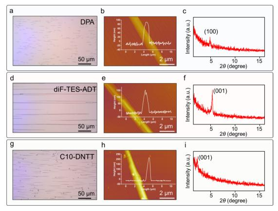
Fig. 4 (a, d and g) OM images of DPA, diF-TES-ADT, and C10-DNTT nanowire arrays with consistent orientation on the m-plane sapphire substrate. (b, e and h) AFM images of DPA, diF-TES-ADT, and C10-DNTT nanowires with smooth surfaces on the m-plane sapphire substrate. (c, f and i) GIXRD images of DPA, diF-TES-ADT, and C10-DNTT on the m-plane sapphire substrate
