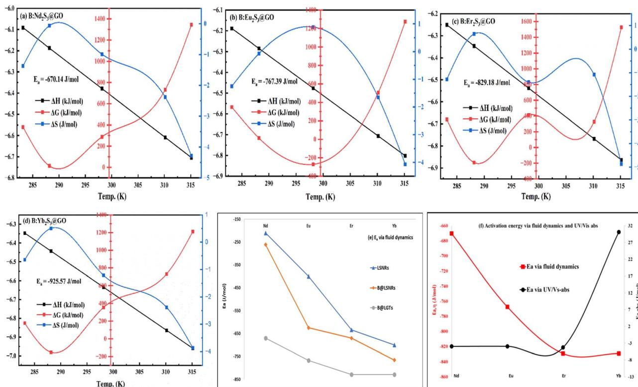
Fig. 21 (a–d) For B@LGTs,  $dH$  linearly decreased while  $dG$  and  $dS$  oppositely vary upon release of heat content on increasing temperature with reorientations and (e)  $E_a$  for photocatalysis. (f)  $E_a$  calculated from fluid dynamics and UV/vis-abs.
