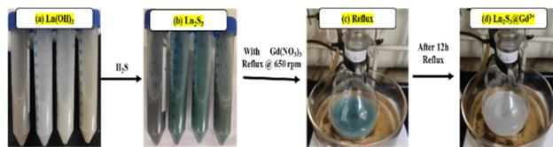
Fig. 3 LSNR doping with  $Gd^{3+}$  for B@LSNR synthesis.
