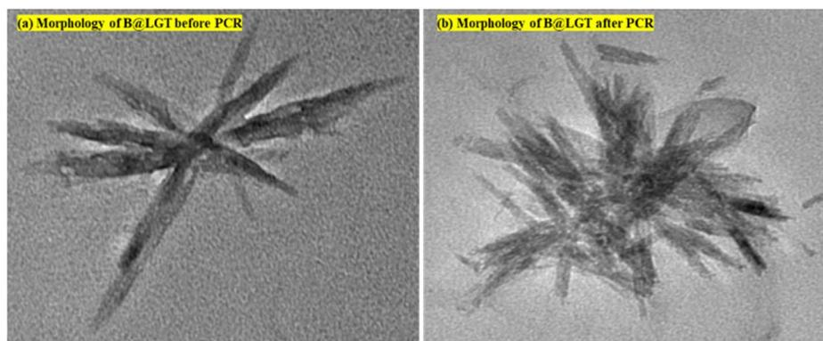
Fig. 30 (a and b) HR-TEM images of B@LGT elucidating the stable morphology before and after the PCR of the pollutants.
