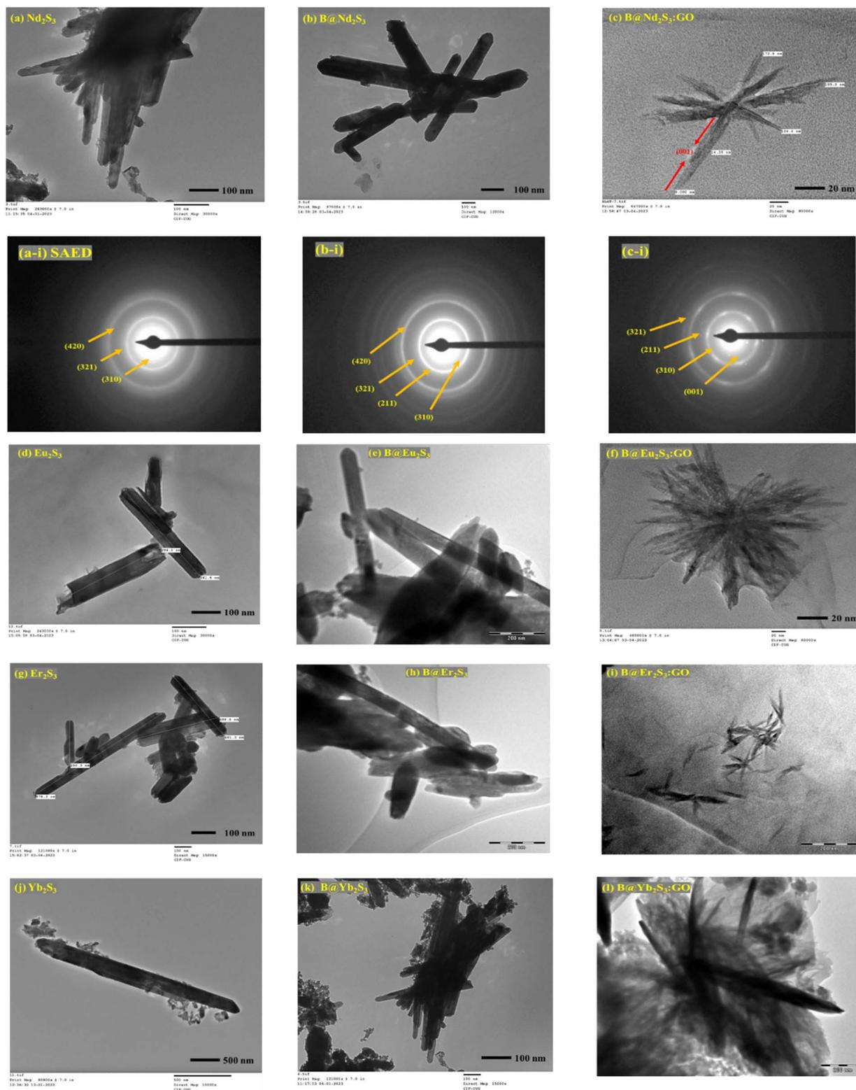
Fig. 9 HR-TEM images of (a–c)  $\text{Nd}_2\text{S}_3$ ,  $\text{B@Nd}_2\text{S}_3$ , and  $\text{B@Nd}_2\text{S}_3\text{:GO}$  with (a(i), b(i), c(i)) their SAED pattern; (d–f)  $\text{Eu}_2\text{S}_3$ ,  $\text{B@Eu}_2\text{S}_3$ , and  $\text{B@Eu}_2\text{S}_3\text{:GO}$ ; (g–i)  $\text{Er}_2\text{S}_3$ ,  $\text{B@Er}_2\text{S}_3$ , and  $\text{B@Er}_2\text{S}_3\text{:GO}$ . (j–l)  $\text{Yb}_2\text{S}_3$ ,  $\text{B@Yb}_2\text{S}_3$ , and  $\text{B@Yb}_2\text{S}_3\text{:GO}$ , respectively.
