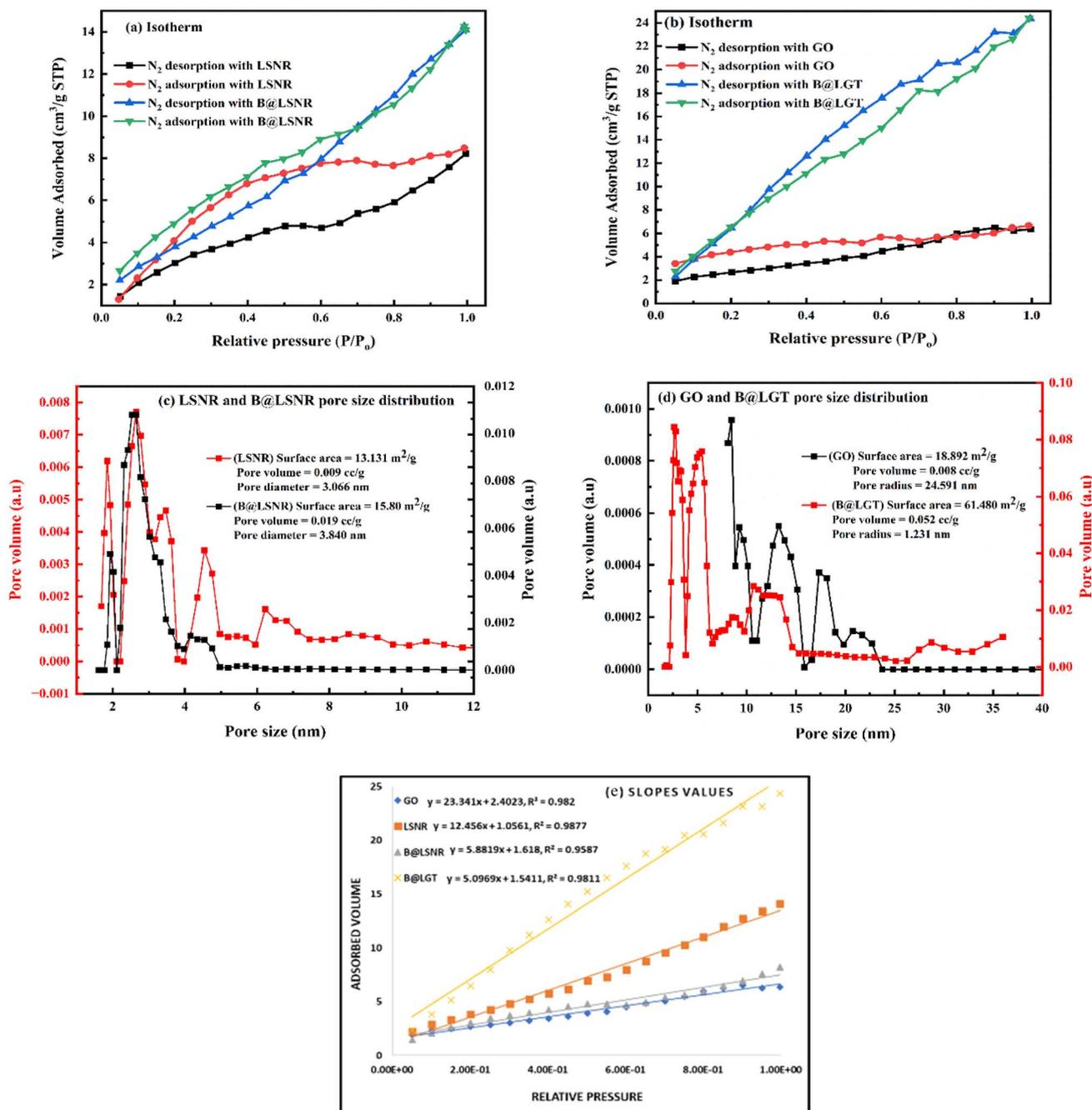
Fig. 6 (a and b) Isotherms and (c and d) pore size of Nd<sub>2</sub>S<sub>3</sub>, B@Nd<sub>2</sub>S<sub>3</sub>, GO, and B:Nd<sub>2</sub>S<sub>3</sub>@GO. (e) Slopes obtained during the adsorption of N<sub>2</sub> by B:Nd<sub>2</sub>S<sub>3</sub>@GO.
