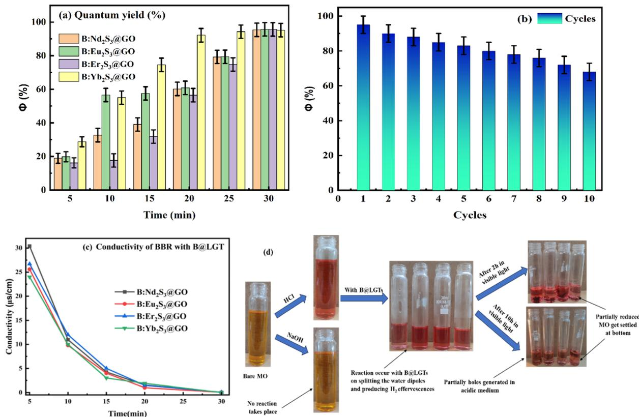
Fig. 32 Spectra elucidating (a)  $\phi$  of BBR, (b) 10 times reusability of B@LGTs, (c) conductivity during the PCR and (d) B@LGTs negligibly undergoing PCR rather than partially adsorbing the MO dye in an acidic medium due to higher potential energy.
