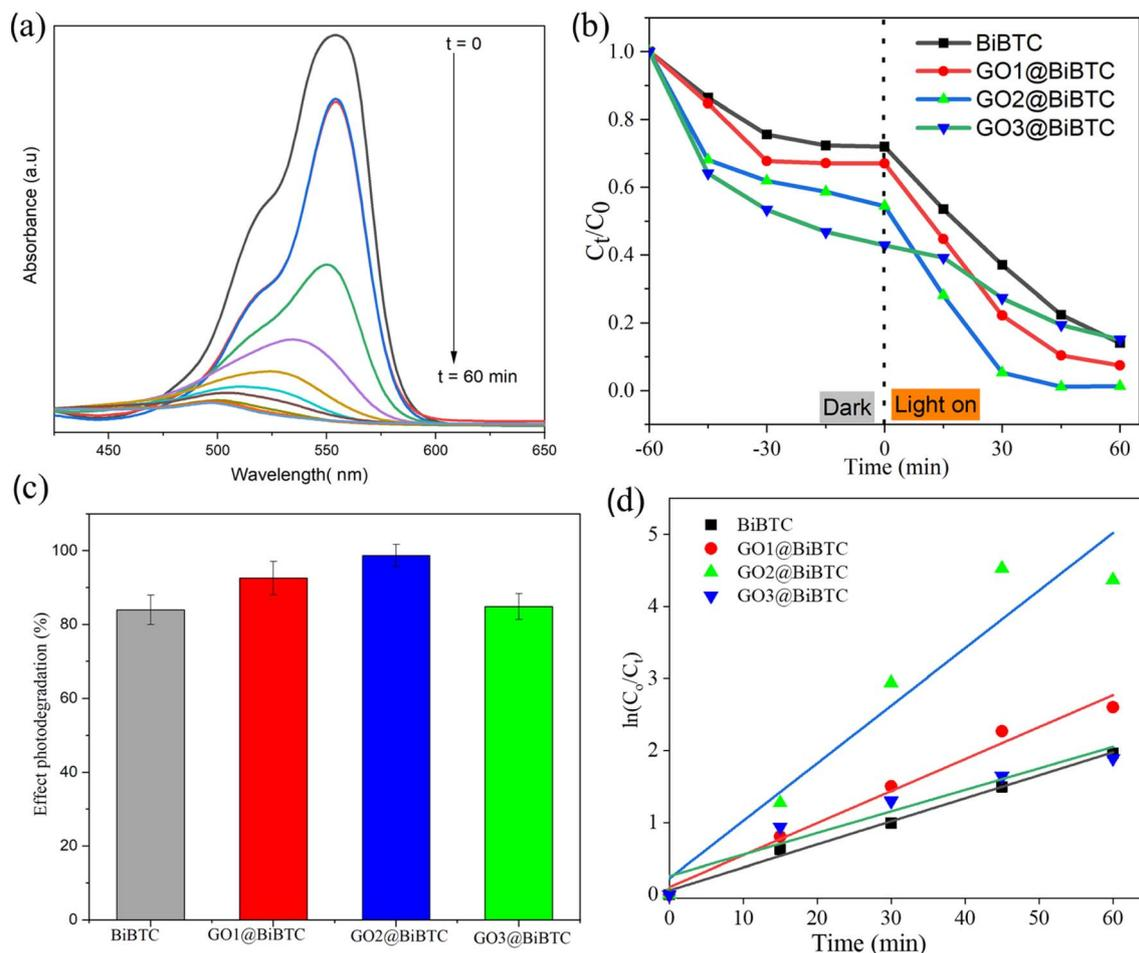
Fig. 12 (a) Absorbance drops under light irradiation, (b)  $C_t/C_0$  vs. irradiation time plots, (c) effect photodegradation-dependent discolorations, and (d)  $\ln(C_0/C_t)$  vs. irradiation time curves using the as-synthesized samples.
