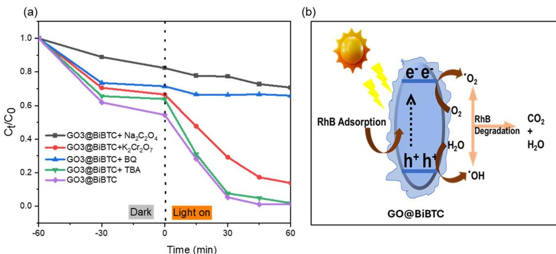
Fig. 16 (a) Photocatalytic RhB degradation without and with radical scavengers and (b) the removal mechanism of RhB by GO@BiBTC MOF heterostructure.
