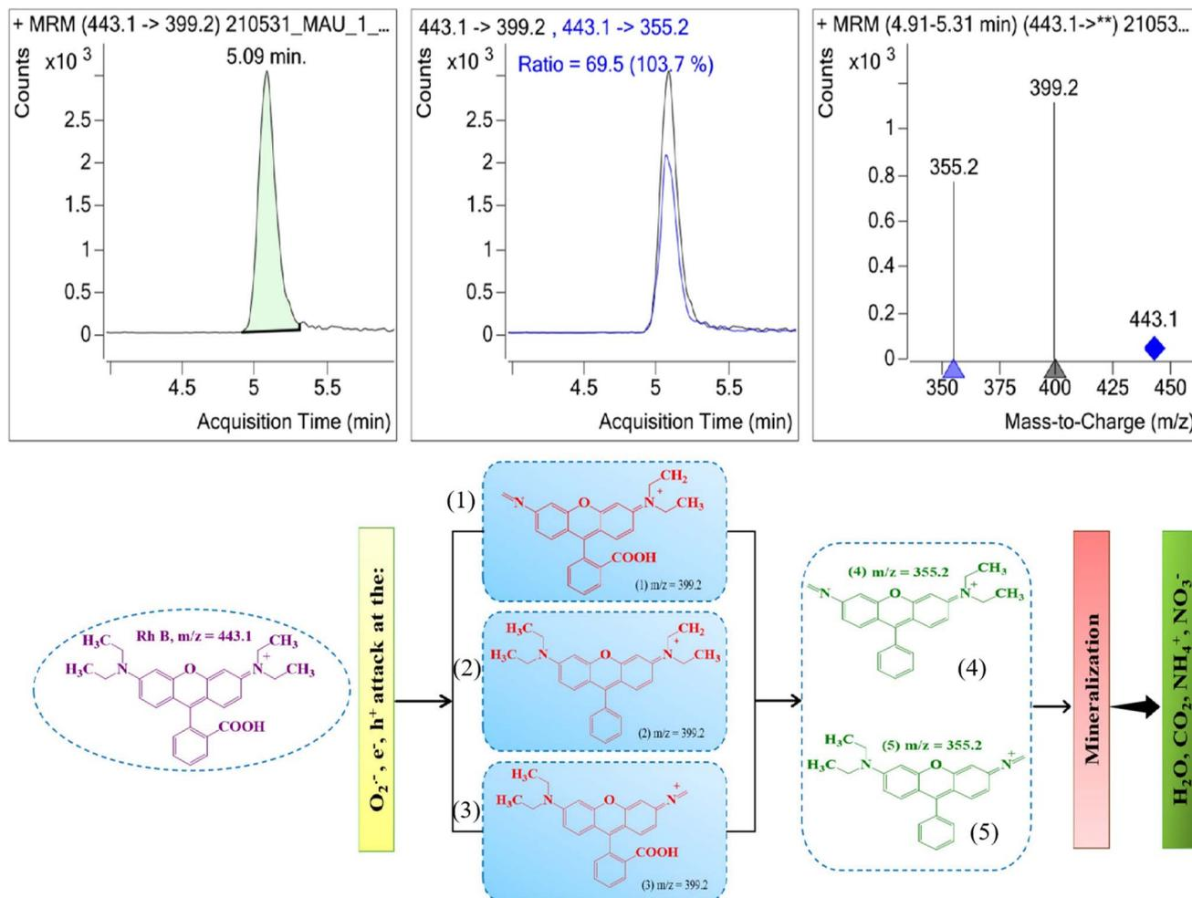
Fig. 17 LC-MS/MS spectroscopy and schematic diagram of plausible degradation of RhB using GO@BiBTC MOF catalyst.
