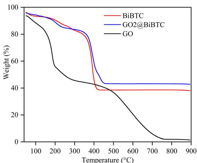
Fig. 8 TGA analyses of the as-synthesized samples.
