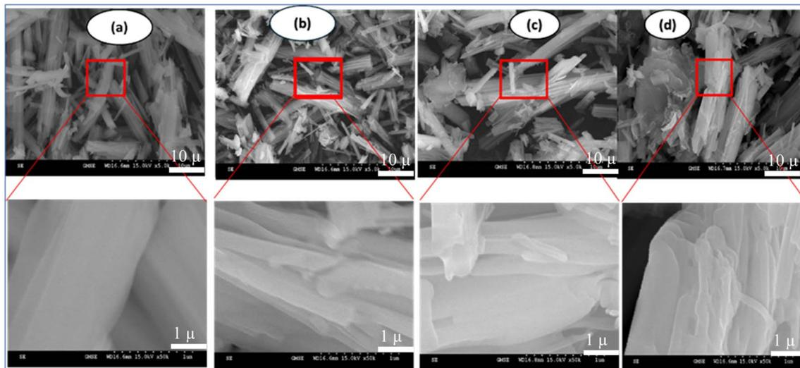
Fig. 4 SEM micrographs of the as-synthesized samples (a) BiBTC, (b) GO1@BiBTC MOF, (c) GO2@BiBTC MOF, (d) GO3@BiBTC MOF photocatalysts.
