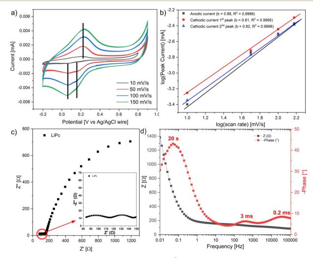
Fig. 7 (a) Cyclic voltammetry of LiPc film with scan rates from 10 to 150 mV  $\rm s^{-1}$  recorded with a three-electrode configuration, (b) dependence of the log(scan rate) vs. log(anodic or cathodic peak currents). (c) Nyquist plot of LiPc film (inset – high-frequency region), and (d) Bode plot of LiPc.
