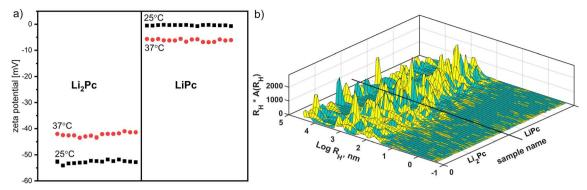
(a) Multiple zeta potential measurements for Li<sub>2</sub>Pc and LiPc water solutions at 25 °C and 37 °C; (b) repeated DLS measurements for Li<sub>2</sub>Pc and LiPc samples at 25 °C.
