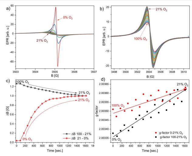
Fig. 5 Successively collected EPR spectra, dwell time 100 ms of (a) nitrogen saturated  $\gamma$ -LiPc; (b) oxygen saturated  $\gamma$ -LiPc sample; (c) peak-topeak linewidth changes in time during desaturation of the atmosphere with  $N_2$  (red circles) and second experiment with  $O_2$  (black squares); and (d) g-factor changes during experiment described in the case shown in Fig. 4c.
