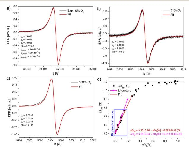
Fig. 4 EPR spectra of LiPc: (a) saturated with  $N_2$ ; (b) in air; (c) saturated with  $O_2$ ; (d) peak-to-peak linewidth dependence vs. oxygen concentration of  $O_2/N_2$  mixture. The dependence is almost linear and can be described as follows  $\Delta B_{pp}$  [mG] =  $3.18 \times pO_2$  [%] + 0.028 in the range 0–21% of  $O_2$ ; this corresponds to the partial oxygen pressure range 0–159.6 mmHg or 0–21.3 kPa. The magenta line is the data from ref. 24 and 25.
