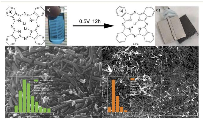
Fig. 1 (a) Chemical structure of dilithium phthalocyanine  $-\text{Li}_2\text{Pc}$ ; (b) diluted  $\text{Li}_2\text{Pc}$  in acetonitrile; (c) chemical structure of lithium phthalocyanine -LiPc; (d) platinum electrodes with LiPc (black layer) on one of them; (e) SEM image of  $\gamma$ -LiPc - scale 10  $\mu$ m, inset - crystal width statistic; and (f) SEM image of LiPc - scale 50  $\mu$ m, inset - crystal length statistics.
