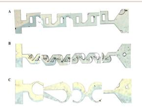
Fig. 7 Mixing efficiency of micromixers using dyes showing T-junction of inlets, the first, last micromixer units and the reaction microchambers of (A) F-shape, (B) Tesla (J)-shape and (C) 8-shape micromixers.
