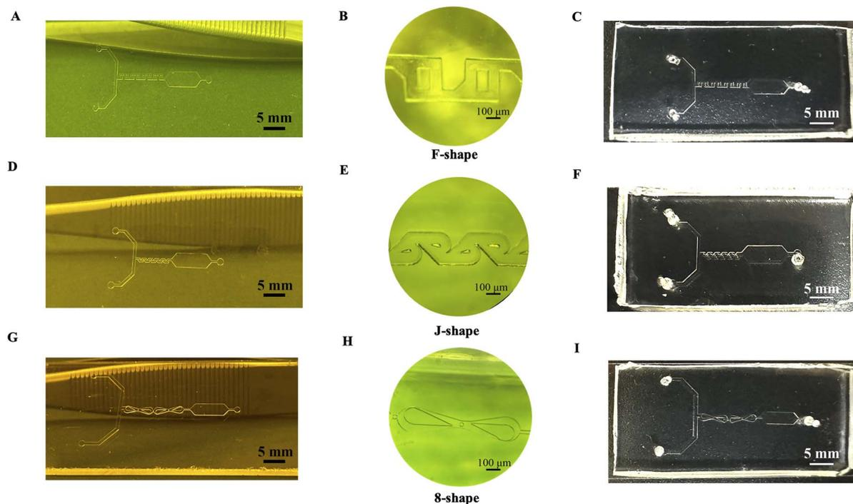
Fig. 4 Microscopic and overall structures of (A and B) F-shape, (D and E) Tesla (J) shape, and (G and H) 8-shape micromixers. (C, F and I) fabricated microfluidic chips with different micromixer designs.
