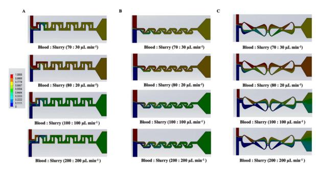
Fig. 6 2D Simulations of all three micromixer types: (A) F-shape, (B) Tesla (J)-shape and (C) 8-shape.
