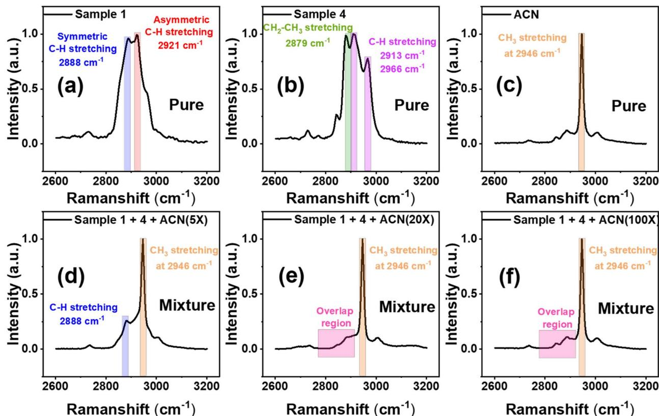
Fig. 2 Impact of ACN solvent on pure VOC mixture between S1 and S4. The Raman spectrum of (a) pure VOC sample S1 *i.e.* 2-nonanone, (b) pure VOC sample S4 *i.e.* 3-methyl-butanoic-acid, and (c) pure acetonitrile (ACN) solvent. Raman spectrum of VOC and ACN mixture with (d) ACN solvent diluted 5 $\times$  (20%), (e) ACN solvent diluted 20 $\times$  (5%), and (f) ACN solvent diluted 100 $\times$  (1%).
