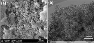
Fig. 2 Elemental microscopy of diamond nanoparticles: (a) SEM; (b) TEM.
