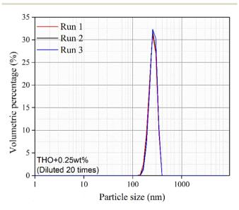
Fig. 5 DLS analysis of diamond/THO nanofluids
