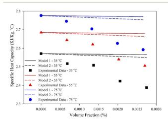
Fig. 9 Comparison of experimental SHC with Model 1 and 2.
