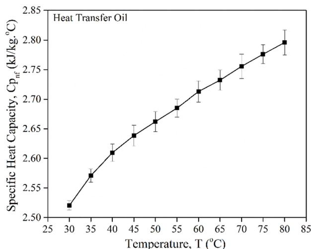
Fig. 1 Repetition of experimental specific heat capacity.
