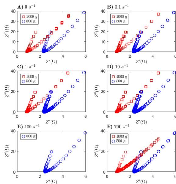
Fig. 8 Impedance in  $\Omega$  as a function of (A)  $0 \text{ s}^{-1}$ , (B)  $0.1 \text{ s}^{-1}$ , (C)  $1 \text{ s}^{-1}$ , (D)  $10 \text{ s}^{-1}$ , (E)  $100 \text{ s}^{-1}$  and (F)  $700 \text{ s}^{-1}$  shear rate for  $1000\text{g}$  GO (red) and  $500\text{g}$  GO (blue). No data was collected for  $1000\text{g}$  GO at  $100 \text{ s}^{-1}$ .
