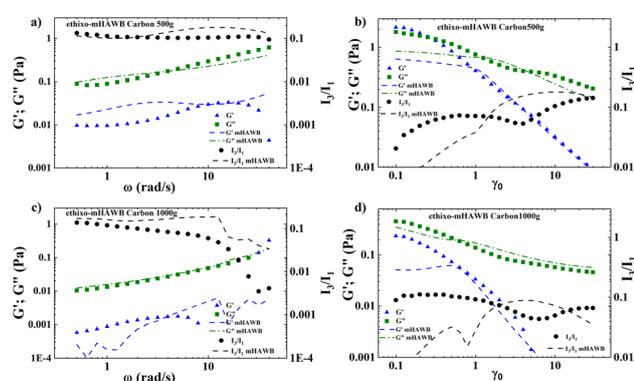
Fig. 4 Ethixo-mHAWB SAOS predictions (discrete point data; dashed lines ethixo-mHAWB predictions) (a) frequency sweep at  $\gamma_0 = 10$ ; and (b) amplitude sweep at  $\omega = 12.6 \text{ rad s}^{-1}$  of the 500g GO suspension; (c) frequency sweep at  $\gamma_0 = 10$ ; and (b) amplitude sweep at  $\omega = 12.6 \text{ rad s}^{-1}$  of the 1000g graphene oxide suspension.
