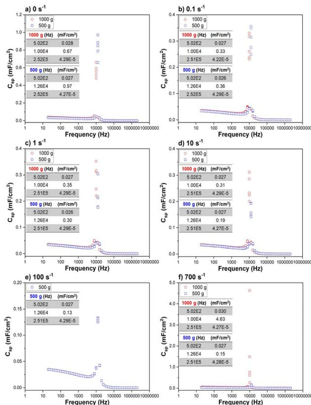
Fig. 9 Specific areal capacitance ( $C_{sp}$ ) as a function of (a)  $0\text{ s}^{-1}$  (b)  $0.1\text{ s}^{-1}$  (c)  $1\text{ s}^{-1}$  (d)  $10\text{ s}^{-1}$  (e)  $100\text{ s}^{-1}$  (f)  $700\text{ s}^{-1}$  shear rate for 1000g GO (red) and 500g GO (blue). No data was collected for 1000g GO at  $100\text{ s}^{-1}$ .
