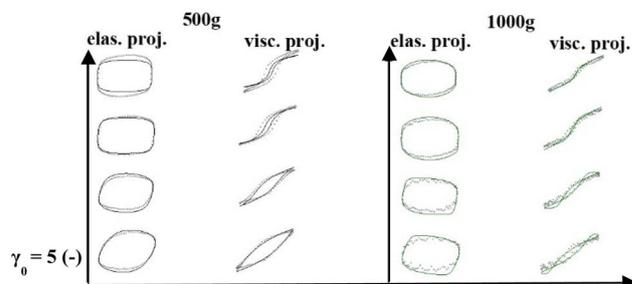
Fig. 5 Ethixo-mHAWB LAOS predictions and LAOS data (discrete points data; dashed lines ethixo-mHAWB predictions) at six different strain amplitudes:  $\gamma_0 = 5, 10, 50$  and  $100$  at  $\omega = 1 \text{ rad s}^{-1}$  for the 500g (black lines) and 1000g (green lines) graphene oxide in water suspensions (\*note  $\sigma$  values are normalized by  $\sigma_{max}$ ).
