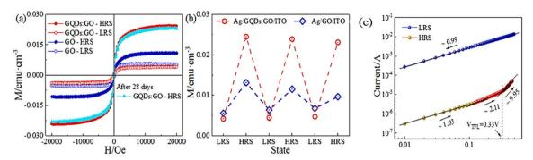
Fig. 21 GQD:GO hybrid film and GO film room-temperature LRS and HRS magnetism. (a) *M-H* curve. (b) RS behaviour causes reversible magnetic moment shifts. (c) Linear fitting of Ag/GQD:GO/ITO device *I-V* curve on log-log scale. Reproduced from ref. 205 with permission from Elsevier. Copyright 2021, Elsevier.
