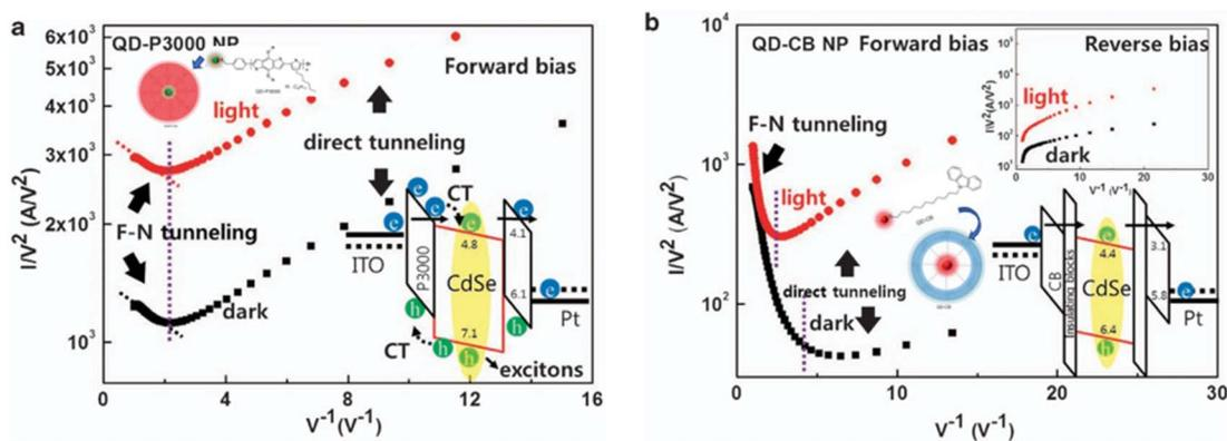
Fig. 3 Fowler–Nordheim (F–N) and direct tunneling models under dark and light conditions with (a) forward conditions of QD-P300 and (b) reverse bias of QD-CB NPs. Energy diagram is shown in the inset. Reproduced from ref. 42 with permission from Springer-Nature.
