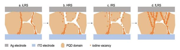
Fig. 5 Schematic of CF formation and annihilation in CsPbI<sub>3</sub> PQD-based device across various states: (a) iLRS; (b) HRS; (c) IRS; and (d) fLRS. Reproduced from ref. 133 with permission from ACS. Copyright 2024, ACS.
