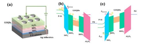
Fig. 15 (a) Pd/Al<sub>2</sub>O<sub>3</sub>/HfO<sub>2</sub>/GOQDs/HfO<sub>2</sub>/SiO<sub>2</sub>/Si charge trapping memory device, (b) programmed state and (c) erased state. Reproduced from ref. 31 with permission from AIP. Copyright 2020, AIP.
