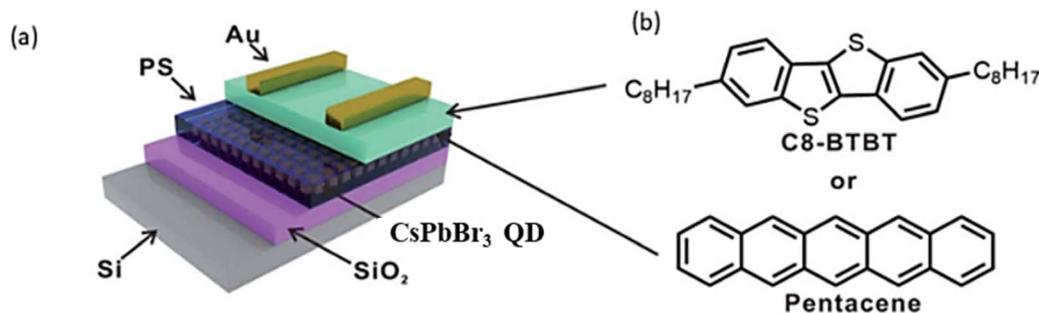
Fig. 8 (a) Diagram showing the structure of CsPbBr<sub>3</sub> quantum dots (QDs) combined with a polystyrene (PS) composite film in field-effect transistor memory devices (FGOFETMs). (b) Molecular structures of pentacene and C8-BTBT. Reproduced from ref. 138 with permission from RSC. Copyright 2020, RSC.
