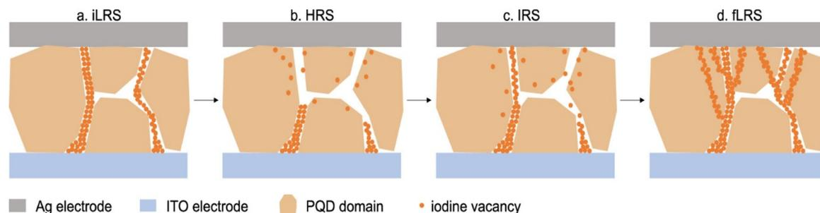
Fig. 5 Schematic of CF formation and annihilation in  $CsPbI_3$  PQD-based device across various states: (a) iLRS; (b) HRS; (c) IRS; and (d) fLRS. Reproduced from ref. 133 with permission from ACS. Copyright 2024, ACS.
