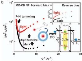
Fig. 3 Fowler–Nordheim (F–N) and direct tunneling models under dark and light conditions with (a) forward conditions of QD-P300 and (b) reverse bias of QD-CB NPs. Energy diagram is shown in the inset. Reproduced from ref. 42 with permission from Springer-Nature.
