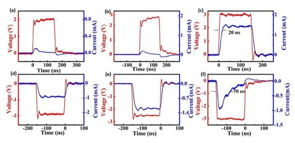
Fig. 18 Results of the switching-speed measurement for the ReRAM device lacking GOQDs. Illustrations include input pulse shapes in red and corresponding output conducting current shapes in blue. The input pulses have amplitudes/widths of (a) 2 V/150 ns, (b) 2.5 V/150 ns, (c) 3 V/150 ns, (d) -2 V/150 ns, (e) -2.5 V/150 ns, and (f) -3 V/150 ns. Reproduced from ref. 20 with permission from RSC. Copyright 2017, RSC
