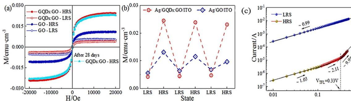
Fig. 21 GQD:GO hybrid film and GO film room-temperature LRS and HRS magnetism. (a)  $M-H$  curve. (b) RS behaviour causes reversible magnetic moment shifts. (c) Linear fitting of Ag/GQD:GO/ITO device  $I-V$  curve on log-log scale. Reproduced from ref. 205 with permission from Elsevier. Copyright 2021, Elsevier.
