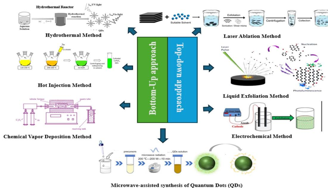
Fig. 4 Different synthesis approaches for quantum dots.
