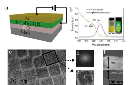
Fig. 6 (a) CsPbBr<sub>3</sub> QD-based WORM setup. (b) Photoluminescence and absorbance of CsPbBr<sub>3</sub> QDs. Daylight and UV light images of CsPbBr<sub>3</sub> QD solution are in the inset. (c-e) TEM images of CsPbBr<sub>3</sub> (f) SEM cross-sectional image of CsPbBr<sub>3</sub> QD-based resistive switching device. Reproduced from ref. 18 with permission from Elsevier. Copyright 2019, Elsevier.
