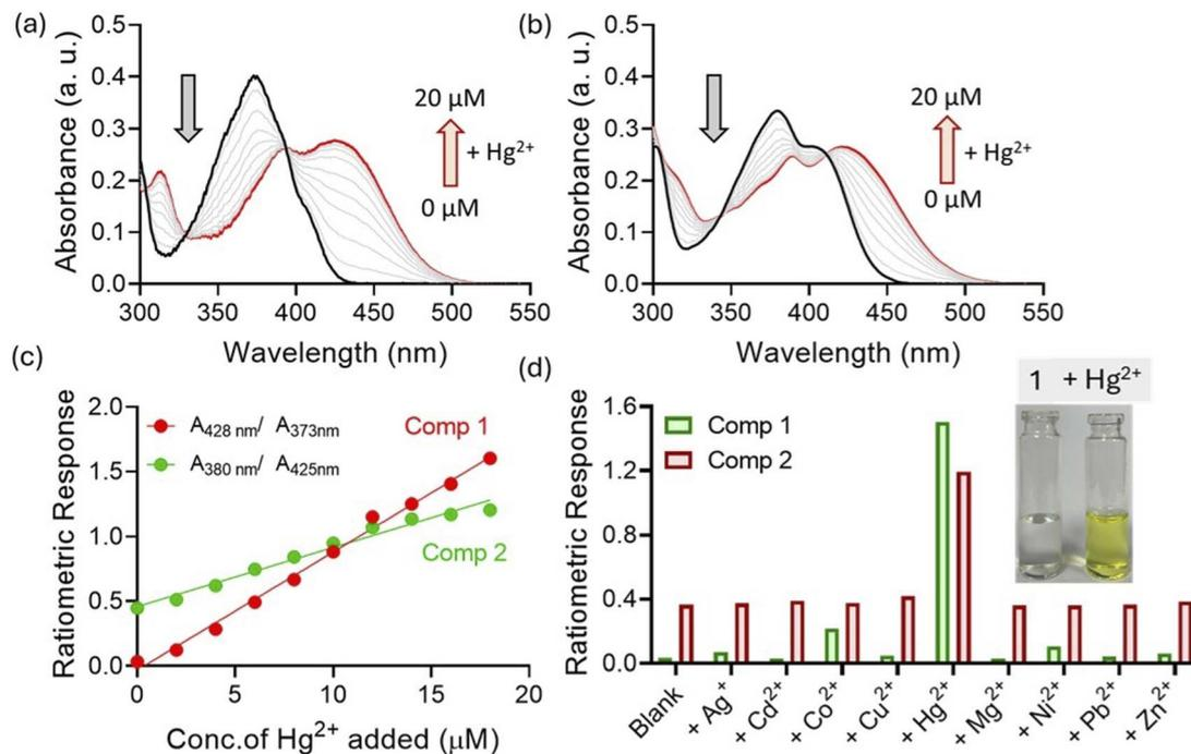
Fig. 4 UV-visible titration of (a) 1 and (b) 2 (10 μM) with Hg<sup>2+</sup> (0–20 μM) in a CH<sub>3</sub>CN medium. (c) Ratiometric responses of 1 and 2 (10 μM) towards Hg<sup>2+</sup> ions (0–20 μM) in a CH<sub>3</sub>CN medium. (d) Ratiometric responses of 1 and 2 (10 μM) in the presence of various metal ions (25 μM) in a CH<sub>3</sub>CN medium [each experiment was independently performed thrice for reproducibility].
