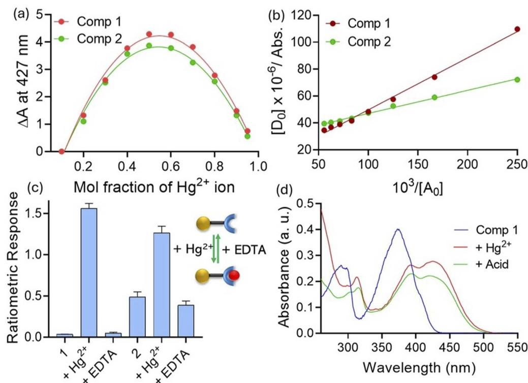
Fig. 6 (a) Job's plot of compounds 1 and 2 in the presence of  $\text{Hg}^{2+}$  ions. (b) Determination of binding constants of compounds 1 and 2 with  $\text{Hg}^{2+}$  ions. (c) Recovery experiment with EDTA showing the reversible interaction of 1 and 2. (d) UV-visible spectra of 1 (10  $\mu\text{M}$ ) with different  $\text{Hg}^{2+}$  salts (25  $\mu\text{M}$ ) in a  $\text{CH}_3\text{CN}$  medium [each experiment was independently performed thrice for reproducibility].
