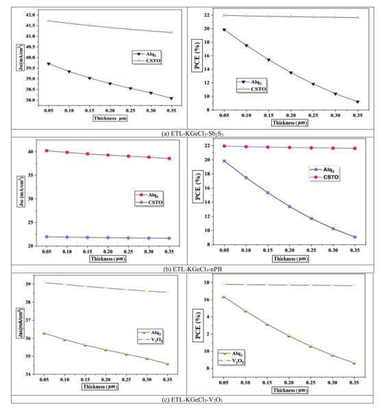
Fig. 6 Effect of ETL thickness.
