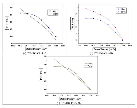
Fig. 11 Effect of absorber defects.
