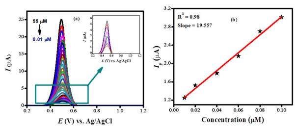
Fig. 6 (a) SWVs of various concentrations (0.01–55  $\mu$ M) of bromothymol blue obtained at NH<sub>2</sub>-fMWCNTs/TiO<sub>2</sub>/GCE in PBS of pH 7.0; (b) calibration plot of bromothymol blue.
