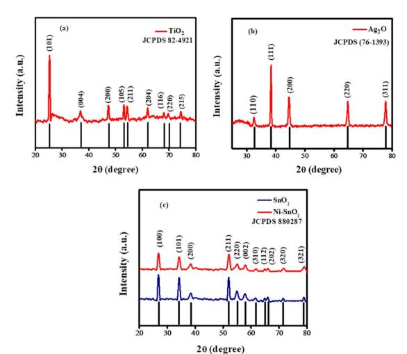
Fig. 1  $\,$  X-ray diffractograms of (a) TiO $_2$  NPs (b) Ag $_2$ O NPs and (c) both doped and undoped SnO $_2$  NPs.
