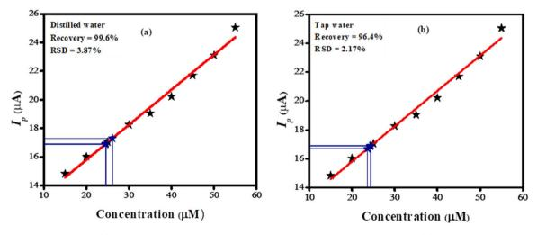
Fig. 7 Calibration plot showing (a) recovery of 25  $\mu$ M spiked amount of bromothymol blue in distilled water; (b) recovery of 25  $\mu$ M spiked amount of bromothymol blue in tap water.
