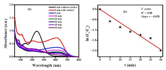
Fig. 8 (a) UV-Vis spectra showing time based decrease in concentration of bromothymol blue dye due to photocatalytic breakdown by Ag<sub>2</sub>O NPs; (b) plot of  $\ln \frac{C_t}{C_0}$  vs. t using UV-Vis spectroscopic data of the photocatalytic breakdown of bromothymol blue.
