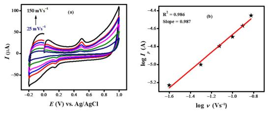
Fig. 4 (a) Cyclic voltammograms showing the impact of the scan rate on the oxidative peak current intensity of 10 μM bromothymol blue in PBS electrolyte of pH 7.0; (b) plot of the log of peak current of bromothymol blue as a function of log of scan rate
