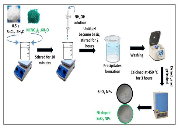
Scheme 3 Protocol for the synthesis of doped and undoped SnO<sub>2</sub> NPs using coprecipitation method.
