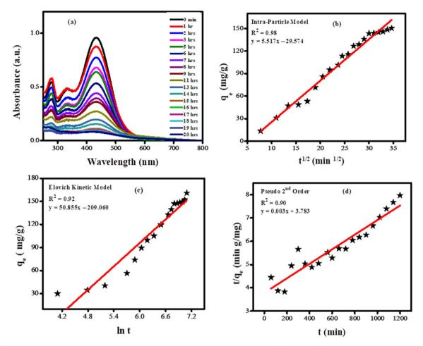
Fig. 11 (a) UV-Vis spectra showing adsorption of bromothymol blue dye over Ni doped SnO<sub>2</sub> NPs; (b) plot according to intraparticle kinetic model; (c) Elovich kinetic model; (d) pseudo second order kinetic model
