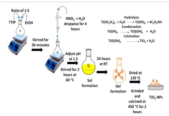
Scheme 1 Sol-gel method for the synthesis of TiO<sub>2</sub> NPs.
