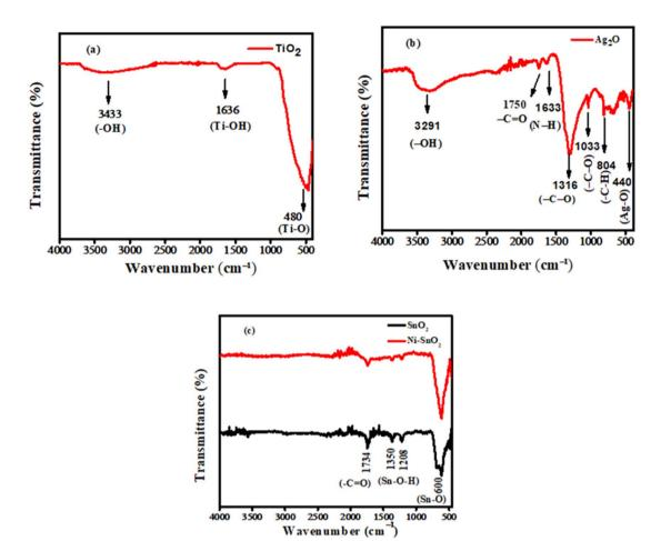
Fig. 2 The FTIR spectra of the synthesized (a)  $TiO_2$  NPs (b)  $Ag_2O$  NPs, and (c)  $SnO_2$  along with Ni-doped  $SnO_2$  NPs.
