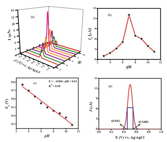
Fig. 5 (a) SWVs of  $10 \mu M$  bromothymol blue obtained by using NH<sub>2</sub>-fMWCNTs/TiO<sub>2</sub>/GCE in PBS solutions of different pH (3–11) at a scan rate of  $100 \text{ mV s}^{-1}$ ; (b) plot of  $I_p$  of bromothymol blue vs. pH of the media; (c) plot of  $E_p$  of bromothymol blue vs. pH of the solutions; (d) FWHM calculated from voltammogram recorded at the modified GCE in medium of pH 7.0.
