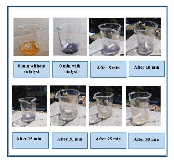
Fig. 10 Photocatalytic degradation of bromothymol blue dye under direct sunlight.
