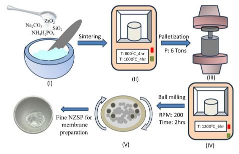
Fig. 1 Schematic depicting a five-step synthesis process of Na<sub>3</sub>Zr<sub>2</sub>Si<sub>2</sub>PO<sub>12</sub> (NZSP)
