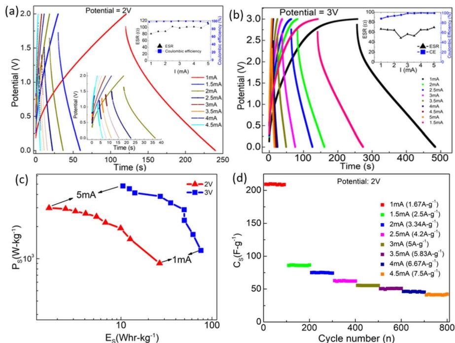
Fig. 9 GCD plots for different currents at operating voltages of (a) 2 V and (b) 3 V, (c) Ragone plot for supercapacitors operating at 2 V and 3 V. (d)  $C_s$  vs. cycle number for different discharge currents at 2 V.
