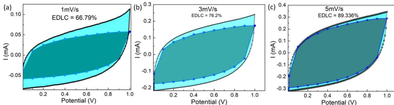
Fig. 10 For the cells with SA  $\sim 1800 \text{ m}^2 \text{ g}^{-1}$  and AN  $\sim 3 \mu\text{L cm}^{-2}$ , the plots depicting EDLC contribution in capacitance for (a)  $1 \text{ mV s}^{-1}$ , (b)  $3 \text{ mV s}^{-1}$ , and (c)  $5 \text{ mV s}^{-1}$ . The shaded region within the actual CV represents the electric double-layer contribution in total capacitance.
