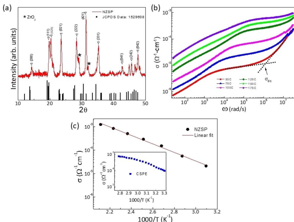
Fig. 3 (a) X-ray diffraction of the as-prepared NZSP along with JCPDS data (card number: 1529608); (b) conductivity vs. frequency plot of pristine NZSP pallet at different temperatures; (c) temperature dependence of conductivity for pristine NZSP pallet and CSPE membrane in the inset.
