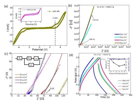
Fig. 6 (a) Cyclic voltammetry (100 mV s $^{-1}$ ) for CSPE membrane with and without AN addition. (b) Nyquist plot of the device, (c) Nyquist plots on an extended scale with corresponding equivalent circuit; (d) GCD plots of devices fabricated with varying amounts of acetonitrile at the electrode–electrolyte interface. (Inset) ESR and coulombic efficiency vs. amount of AN. These results correspond to supercapacitors with activated carbon electrodes of SA  $\sim$ 1000 m $^2$  g $^{-1}$ .
