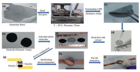
Fig. 2 Preparation steps for the composite solid polymer electrolyte (CSPE) membrane and the supercapacitor fabrication: (a) composite electrolyte slurry (b) hot press for CSPE membrane preparation, (c) flexible CSPE membrane, (d) solvent addition at the CSPE surface, (e and f) supercapacitor components, (g and h) schematic diagram and the supercapacitor in sandwich geometry, and (i) final laminated supercapacitor.
