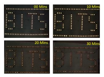
Fig. 12 Five-cells linked in series make a glowing LED circuit (8 V).
