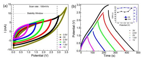
Fig. 8 (a) CV (b) GCD curves for optimized supercapacitor (SA  $\sim$  1800 m<sup>2</sup> g<sup>-1</sup> and AN  $\sim$  3  $\mu$ L cm<sup>-2</sup>) at different operating voltages.
