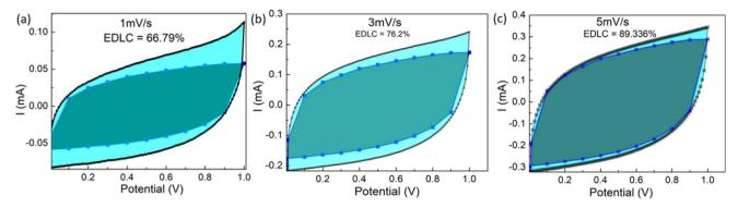
Fig. 10 For the cells with SA  $\sim$ 1800 m<sup>2</sup> g<sup>-1</sup> and AN  $\sim$  3  $\mu$ L cm<sup>-2</sup>, the plots depicting EDLC contribution in capacitance for (a) 1 mV s<sup>-1</sup>, (b) 3 mV s<sup>-1</sup>, and (c) 5 mV s<sup>-1</sup>. The shaded region within the actual CV represents the electric double-layer contribution in total capacitance.
