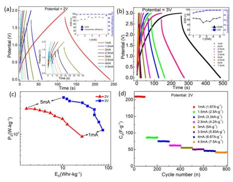
Fig. 9 GCD plots for different currents at operating voltages of (a) 2 V and (b) 3 V, (c) Ragone plot for supercapacitors operating at 2 V and 3 V. (d)  $C_s$  vs. cycle number for different discharge currents at 2 V.
