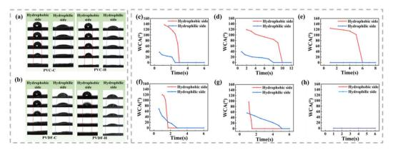
Fig. 4 (a and b) Changes in the shape of water droplets on composite fabrics with different hydrophobic layers prepared using an electrospraying time of 3 h. (c-e) For PVC, the changes in WCA over time are shown for cotton, hemp, and modal, from left to right. (f-h) For PVDF, the changes in WCA over time are shown for cotton, hemp, and modal, from left to right.
