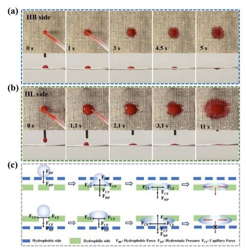
Fig. 7 Wetting behavior of ink droplets on (a) HL and (b) HB surfaces as viewed from the top and side, respectively (c) Schematic diagram of directional water transport mechanism (HL represents the hydrophilic side and HB represents the hydrophobic side).
