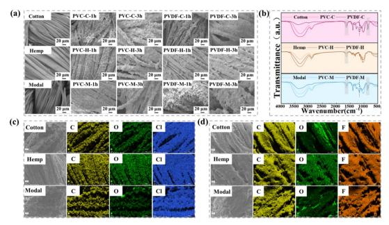
Fig. 2 (a) SEM images of the fabrics prepared with different electrospraying times. (b) FTIR spectra of the fabrics after 3 h of electrospraying. EDS spectra of the fabrics coated with (c) PVC and (d) PVDF.
