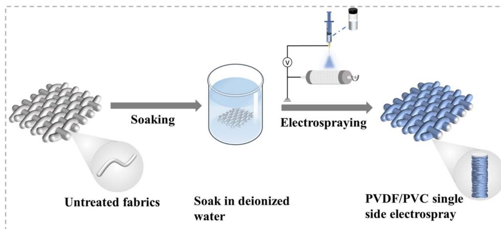
Fig. 1 Illustration of the process used for preparing and analyzing unidirectional moisture-conducting composite fabrics.
