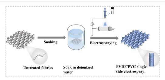
Fig. 1 Illustration of the process used for preparing and analyzing unidirectional moisture-conducting composite fabrics.
