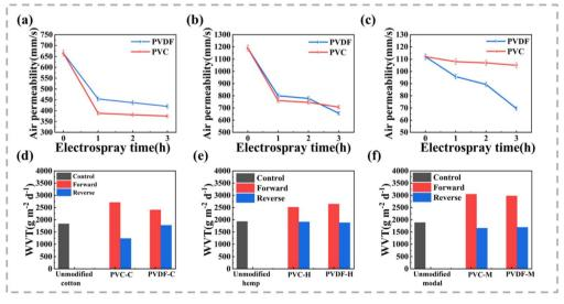
Fig. 8 (a-c) Air permeability of composite fabrics at different electrospraying times, (a) cotton, (b) hemp and (c) modal. (d-f) WVT rate of composite fabrics at 3 h of electrospraying, (d) cotton, (e) hemp and (f) modal.
