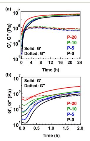
Fig. 4 (a) Isothermal time-resolved rheology data measured at 170 °C for 24 h. (b) Expanded data within initial 2 h. The translucent circle represents the cross-point of G' and G''.
