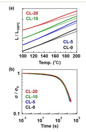
Fig. 6 (a) Temperature-ramp creep data. The Y-axis represents the sample length (L) normalized by the length at 100 °C ( $L_{100^{\circ}\text{C}}$ ). The dotted line indicates the approximated straight line extrapolated from low temperature. (b) Stress-relaxation spectra at 180 °C. The Y-axis represents the stress ( $\sigma$ ) normalized by the initial stress ( $\sigma$ <sub>0</sub>).
