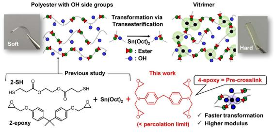
Fig. 1 The molecular design for self-transformation of thermoplastic polyesters into vitrimers. Effects of 4-epoxy as the pre-crosslink in the initial polyester on the transformation performance is investigated in this work.
