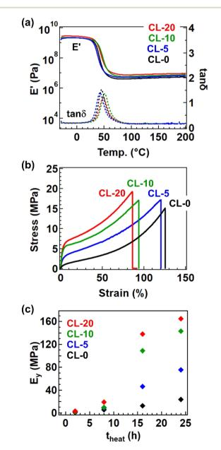
Fig. 5 Physical properties of the cross-linked samples after heating at 170 °C for 24 h. (a) Temperature-sweep rheology data and (b) tensile properties. (c) Variation of  $E_{\rm V}$  as a function of heating time ( $t_{\rm heat}$ ).
