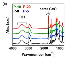
Fig. 2 FT-IR spectra for polyesters with various fractions of 4-epoxy at (a) the SH signal region, (b) the epoxy signal region, and (c) the whole region. In (a) and (b), the spectra of starting monomers (2-SH, 2-epoxy, and 4-epoxy) are also provided for comparison. The inverse triangle represents the characteristic signals from SH and epoxy groups. In (c), the spectra are normalized by C=O signal of ester bonds.
