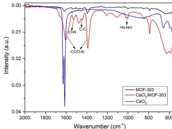
Fig. 7 FTIR spectra of MOF-303, CaCl<sub>2</sub>/MOF-303 and CaCl<sub>2</sub>.
