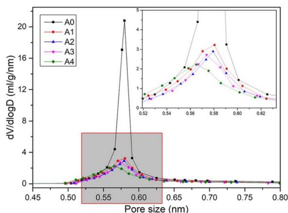
Fig. 4 Pore size distribution curves of MOF-303 and CaCl<sub>2</sub>/MOF-303 composites.
