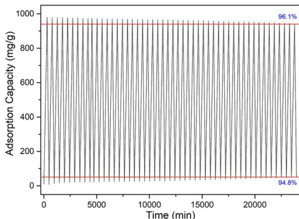
Fig. 13 Cyclic adsorption and desorption of  $\text{CaCl}_2/\text{MOF-303}$  (3).
