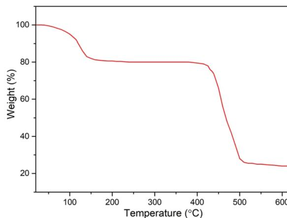
Fig. 8 Thermogravimetric curve of the CaCl<sub>2</sub>/MOF-303 composite.
