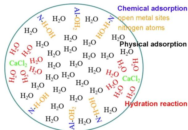
Fig. 12 Schematic diagram of water adsorption mechanism of CaCl<sub>2</sub>/MOF-303 composites.
