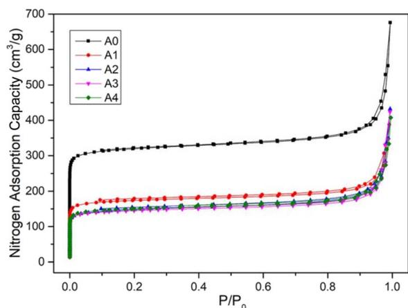
Fig. 3 Nitrogen adsorption curves of MOF-303 and CaCl<sub>2</sub>/MOF-303 composites.
