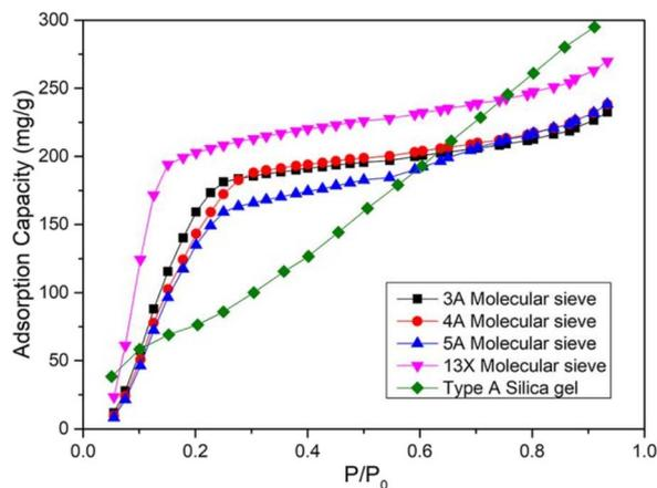
Fig. 10 Water adsorption curves of traditional materials.
