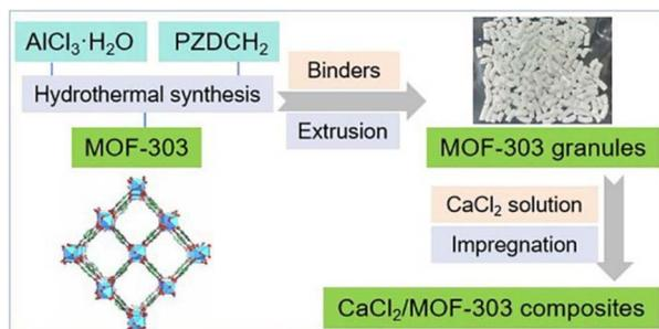
Fig. 1 The preparation diagram of the  $\text{CaCl}_2/\text{MOF-303}$  composite.
