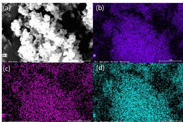
Fig. 6 (a) Total, (b) Al, (c) Ca, and (d) Cl element distribution of CaCl<sub>2</sub>/MOF-303 composite.
