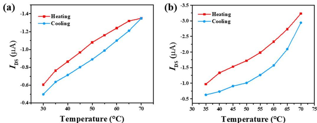
Fig. 4 Temperature dependence of the drain-source current for a 'blank device' (a) and for device B (b) extracted from transfer curves at  $V_G = -30$  V and  $V_{DS} = -10$  V. Channel width  $W = 50$   $\mu\text{m}$ , channel length  $L = 1000$   $\mu\text{m}$ , OSC thickness = 50 nm, and SCO thickness = 50 nm.
