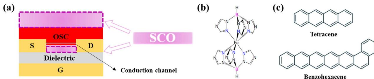
Fig. 1 (a) Schematic of different SCO-OFET configurations using a BG/BC OFET as an example. Molecular structure of (b) the SCO compound [Fe(HB(1,2,4-triazol-1-yl)<sub>3</sub>)<sub>2</sub>] (note that the formal charges of the iron and boron atoms are +2 and –1, respectively) and (c) the OSC compounds (tetracene and benzo[h]hexacene) used in this study.
