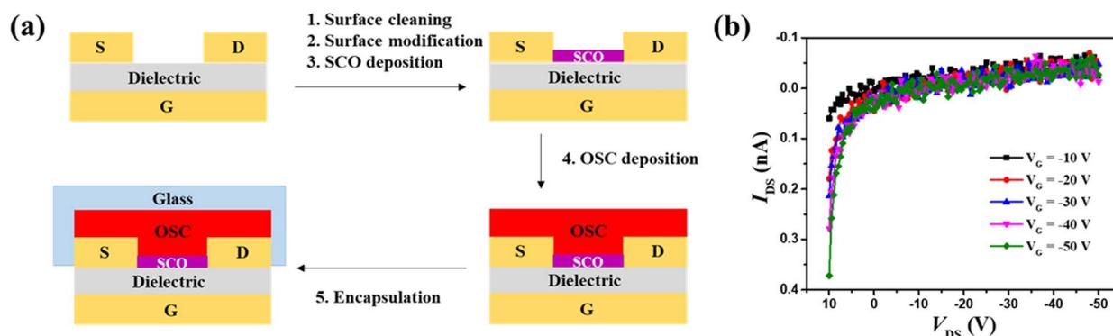
Fig. 2 (a) Process scheme of the BG/BC OFET with the SCO layer between the OSC and the gate dielectric (device A). (b) Representative output characteristics ( $V_G = -10, -20, -30, -40$  and  $-50$  V) of device A (see the transfer characteristic of the same device in Fig. S2a†). Channel width  $W = 50$   $\mu\text{m}$ , channel length  $L = 1500$   $\mu\text{m}$ , OSC thickness = 50 nm, and SCO thickness = 30 nm.
