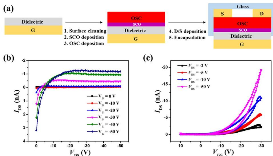
Fig. 3 (a) Process scheme of the BG/TC OFET with the SCO layer positioned between the OSC and the gate dielectric (device B). (b) Output characteristics ( $V_G = 0, -10, -20, -30, -40$  and  $-50$  V) and (c) transfer characteristics ( $V_{DS} = -2, -5, -10$  and  $-50$  V) of device B measured at 45 °C. Channel width  $W = 70$   $\mu\text{m}$ , channel length  $L = 1000$   $\mu\text{m}$ , OSC thickness = 50 nm, and SCO thickness = 50 nm.
