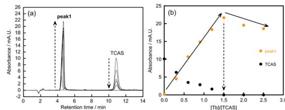
Fig. 5 (a) Chromatograms of the molar ratio method and (b) molar ratio curves between  $[\text{Tb}^{3+}]$  and  $[\text{TCAS}]$  for the Ca-Tb-TCAS system at pH 6.0.  $[\text{Ca}^{2+}] = 20 \mu\text{M}$ ,  $[\text{Tb}^{3+}] = 0-0.10 \text{ mM}$ ,  $[\text{TCAS}] = 40 \mu\text{M}$ ,  $[\text{MES}] = 20 \text{ mM}$ , pH 6.0,  $\lambda = 316 \text{ nm}$ ,  $t = 24$  h,  $60^\circ\text{C}$ .
