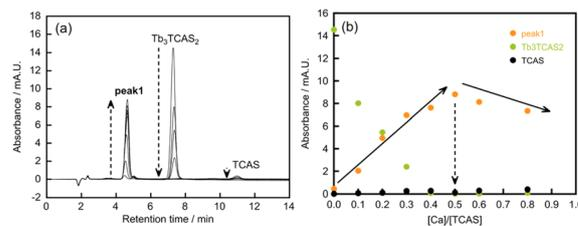
Fig. 4 (a) Chromatograms of the molar ratio method and (b) molar ratio curves between  $[\text{Ca}^{2+}]$  and  $[\text{TCAS}]$  for the Ca-Tb-TCAS system at pH 6.0.  $[\text{Ca}^{2+}] = 0-16 \mu\text{M}$ ,  $[\text{Tb}^{3+}] = 30 \mu\text{M}$ ,  $[\text{TCAS}] = 20 \mu\text{M}$ ,  $[\text{MES}] = 20 \text{ mM}$ , pH 6.0,  $\lambda = 316 \text{ nm}$ ,  $t = 24$  h,  $60^\circ\text{C}$ .
