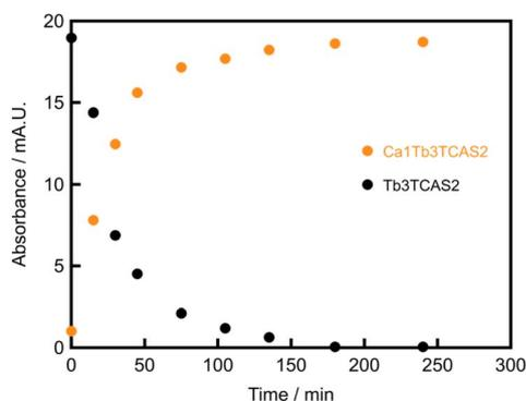
Fig. 8 Time dependence of the height of the HPLC peaks of the  $\text{Ca}_1\text{Tb}_3\text{TCAS}_2$  complex in the mixture of the  $\text{Tb}_3\text{TCAS}_2$  complex and  $\text{Ca}^{2+}$ .  $[\text{Ca}^{2+}] = 0.10$  mM,  $[\text{Tb}_3\text{TCAS}_2] = 0.10$  mM, pH 10 (adjusted with  $\text{NH}_3$ ), 60 °C.
