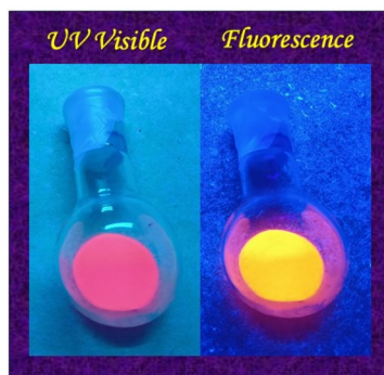
Fig. 16 Silica gel demonstrating a colorimetric and fluorescence response of P1 to \text{Ni}^{2+} ions in a solid medium.
