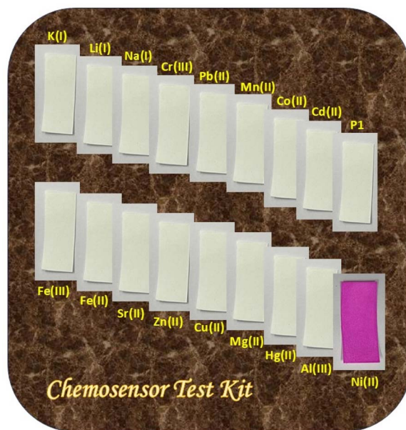
Fig. 15 The chemosensor test kit demonstrating the selective detection of nickel using P1 -coated paper strips.
