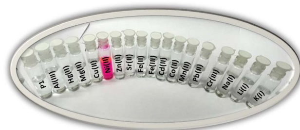
Fig. 2 The observable alterations in color of P1 (10 \mu\text{M} , \text{CH}_3\text{CN} , pH 7.0) following the addition of 1 equivalent of different metal salts.
