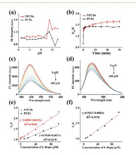
Fig. 3 Influence of (a) pH and (b) detection time on quenching efficiency  $(F_0/F)$ . Fluorescence spectra of (c) NPCDs and (d) PCDs in the presence of L-Dopa at different concentrations. Linear relationship between  $F_0/F$  and L-Dopa concentration in (e) ultrapure water and (f) FBS matrix.
