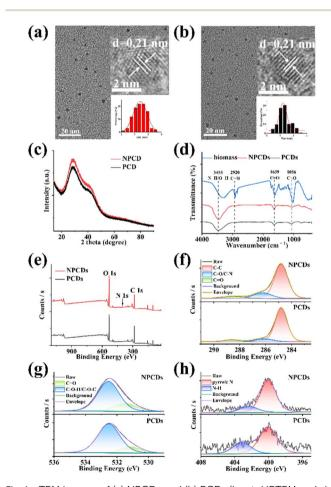
Fig. 1 TEM images of (a) NPCDs and (b) PCDs (inset: HRTEM and size distribution of NPCDs and PCDs). (c) XRD patterns and (d) FTIR spectra of NPCDs and PCDs. (e) XPS full-scan spectrum and high-resolution XPS spectra of (f) C 1s, (g) O 1s and (h) N 1s of NPCDs and PCDs.
