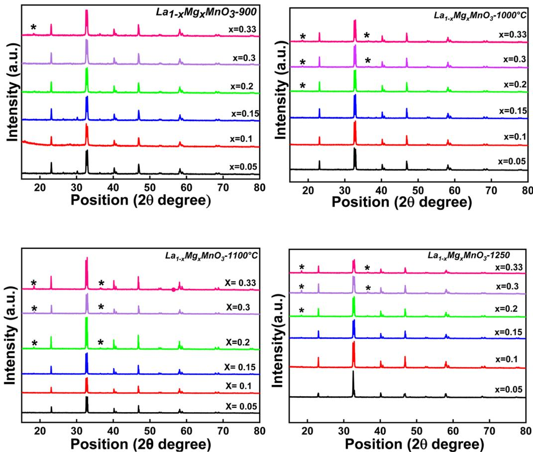
Fig. 1 XRD patterns of LMMO<sub>3</sub> calcined at 900 °C, 1000 °C, 1100 °C and 1250 °C. A regular increase in the intensity of the secondary phase MgMn<sub>2</sub>O<sub>4</sub> is observed.
