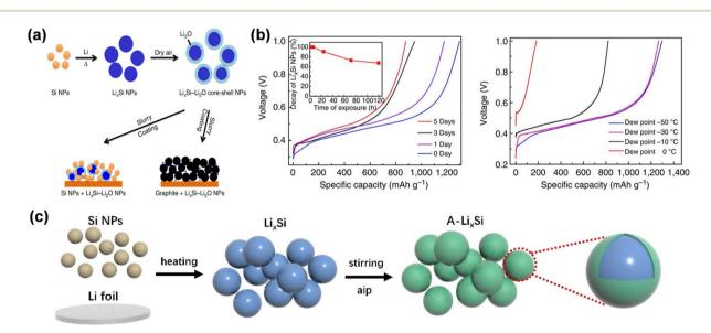
Fig. 9 (a) Schematic diagrams showing Si NPs react with melted Li to form Li<sub>x</sub>Si NPs. (b) The capacity retention of Li<sub>x</sub>Si-Li<sub>2</sub>O NPs exposed to dry air with varying durations and air at different humidity levels (reprinted from ref. 69. Copyright 2014, with permission from Springer Nature). (c) Synthesis process for the Li<sub>x</sub>Al<sub>v</sub>SiO<sub>z</sub>/Li<sub>2</sub>O-coated Li<sub>x</sub>Si (A-Li<sub>x</sub>Si).
