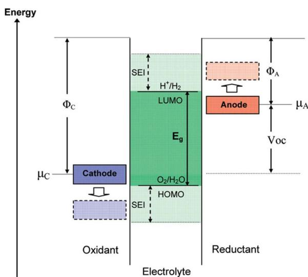
Fig. 3 Schematic open-circuit energy diagram of an aqueous electrolyte.  $\Phi_A$  and  $\Phi_C$  are the anode and cathode work functions.  $E_g$  is the window of the electrolyte for thermodynamic stability (reprinted from ref. 45. Copyright 2009, with permission from ACS Publications).
