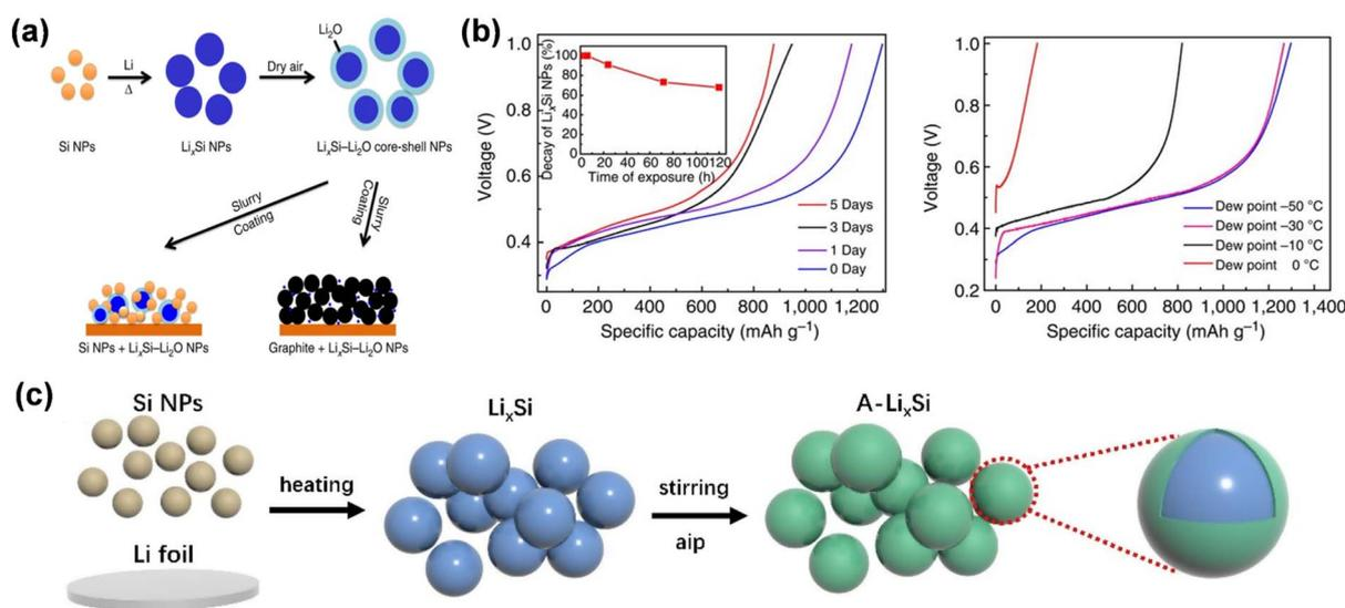
Fig. 9 (a) Schematic diagrams showing Si NPs react with melted Li to form  $\text{Li}_x\text{Si}$  NPs. (b) The capacity retention of  $\text{Li}_x\text{Si-Li}_2\text{O}$  NPs exposed to dry air with varying durations and air at different humidity levels (reprinted from ref. 69. Copyright 2014, with permission from Springer Nature). (c) Synthesis process for the  $\text{Li}_x\text{Al}_y\text{SiO}_z/\text{Li}_2\text{O}$ -coated  $\text{Li}_x\text{Si}$  (A- $\text{Li}_x\text{Si}$ ).
