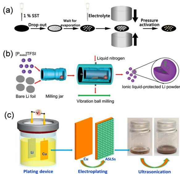
Fig. 11 (a) Schematic illustration of pre-lithiation process on an SiO electrode (reprinted from ref. 67. Copyright 2021, with permission from ACS Publications). (b) Schematic illustration of the ionic liquid-assisted cryomilling preparation process for nanoscaled Li powders (reprinted from ref. 75. Copyright 2019, with permission from Wiley-VCH). (c) Schematic of the fabrication process of the ASLSs (reprinted from ref. 76. Copyright 2021, with permission from Elsevier).
