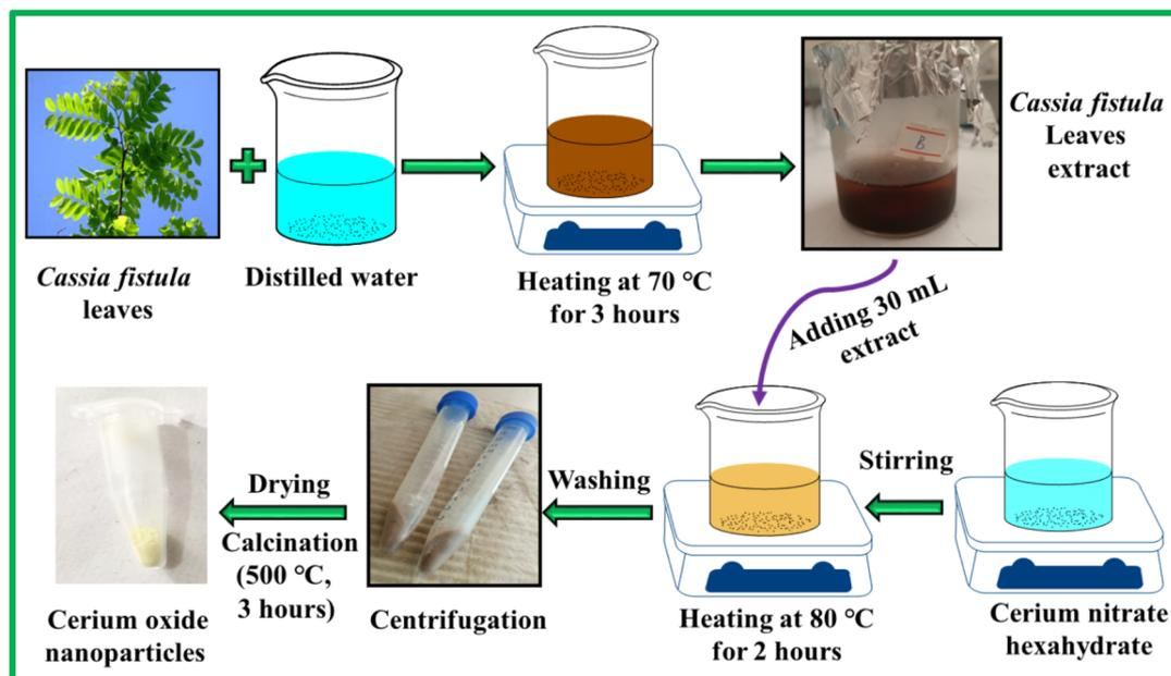
Fig. 1 *C. fistula*-mediated synthesis of CeO<sub>2</sub> NPs.
