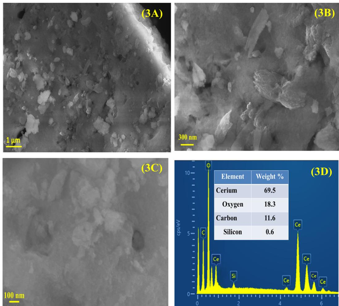
Fig. 3 (A–C) FE-SEM micrographs of CeO<sub>2</sub> captured at various magnifications along with (D) EDX analysis.
