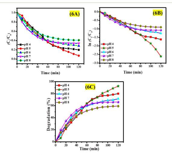
Fig. 6 (A) Graph of  $C_t/C_0$  versus time, (B) kinetic analysis of the photocatalytic degradation of EY in different pH environments, and (C) impact of solution pH on the photocatalytic EY degradation efficiency of CeO2 NPs.
