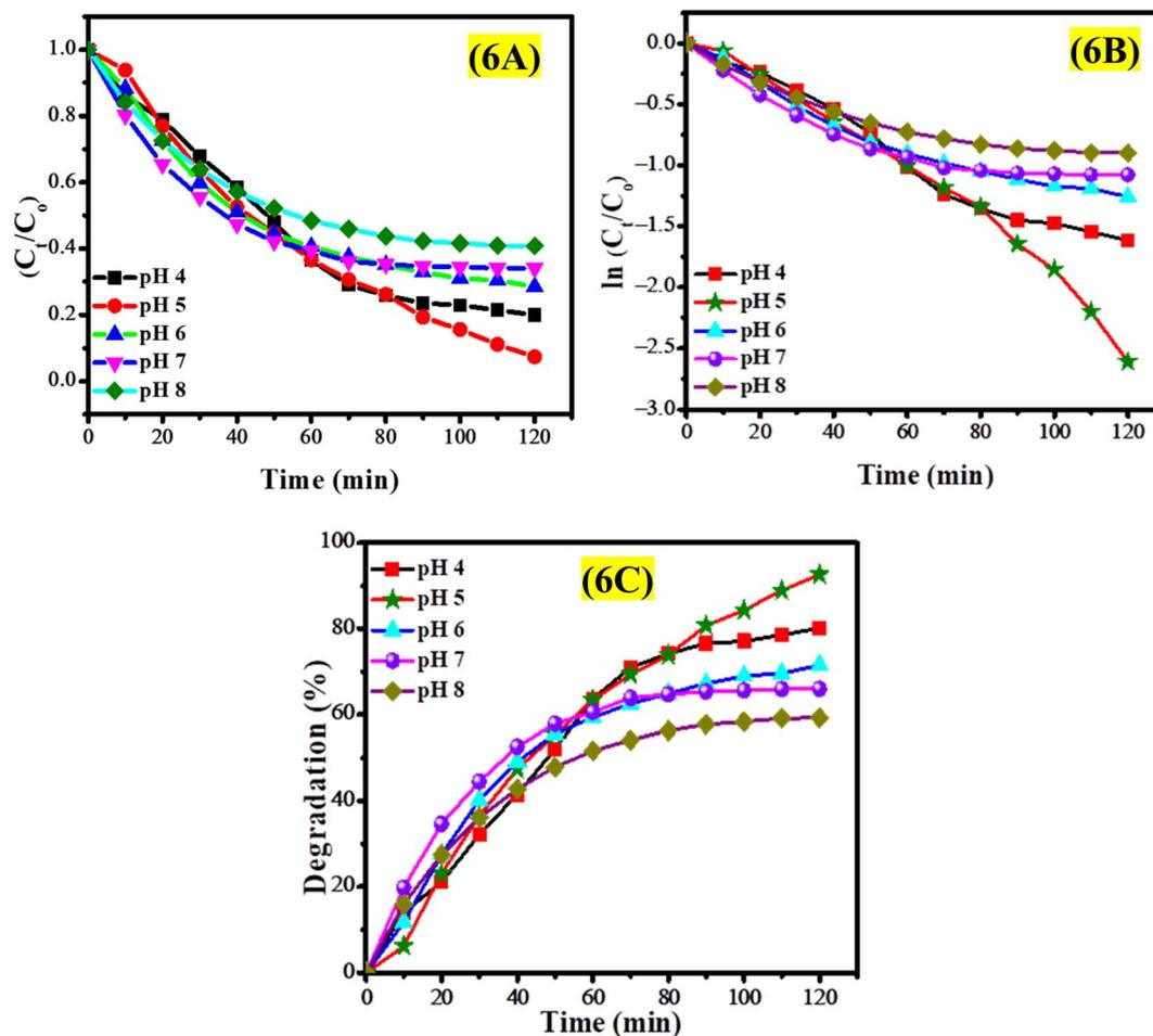
Fig. 6 (A) Graph of  $C_t/C_0$  versus time, (B) kinetic analysis of the photocatalytic degradation of EY in different pH environments, and (C) impact of solution pH on the photocatalytic EY degradation efficiency of  $\text{CeO}_2$  NPs.
