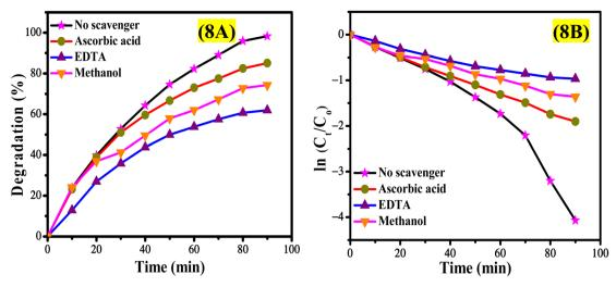
Fig. 8 The influence of the radical scavenger on the (A) degradation percentage and (B) the rate constant of the photocatalytic degradation of EY.
