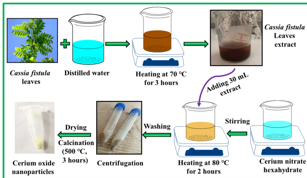
Fig. 1 C. fistula -mediated synthesis of CeO 2 NPs.
