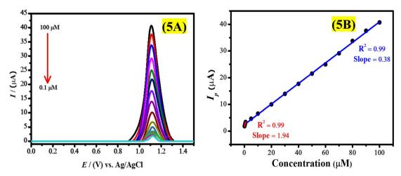
Fig. 5 (A) Voltammetric response of various concentrations of EY using COOH-fMWCNTs/GCE and (B) linear plot using peak current values of 0.1  $\mu$ M to 0.9  $\mu$ M solutions of EY.
