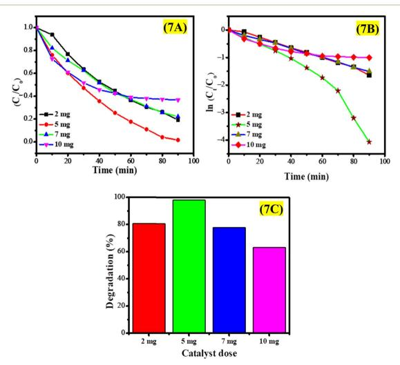
Fig. 7 (A) Graph of  $C_t/C_o$  versus time, (B) kinetic study using pseudo-first-order kinetics, and (C) percentage degradation of EY using different amounts of CeO<sub>2</sub> NPs.
