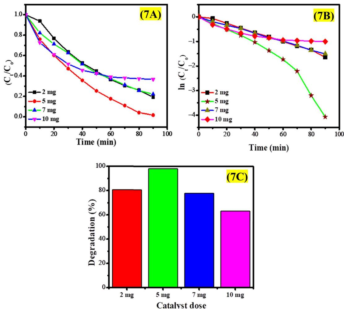
Fig. 7 (A) Graph of  $C_t/C_0$  versus time, (B) kinetic study using pseudo-first-order kinetics, and (C) percentage degradation of EY using different amounts of CeO<sub>2</sub> NPs.
