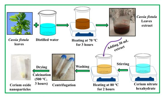
Fig. 1 C. fistula-mediated synthesis of CeO<sub>2</sub> NPs.
