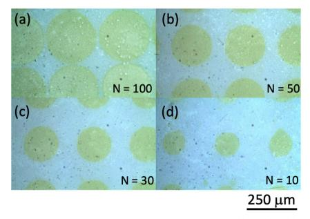
Fig. 12 Optical microphotographs of areas printed using ink 'D' with the number of shots N of (a) 100, (b) 50, (c) 30, and (d) 10. The scale bar length is 250 µm.
