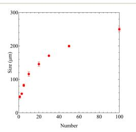
Fig. 13 Shot number dependences of dot size (diameter) when printed using ink 'D'.
