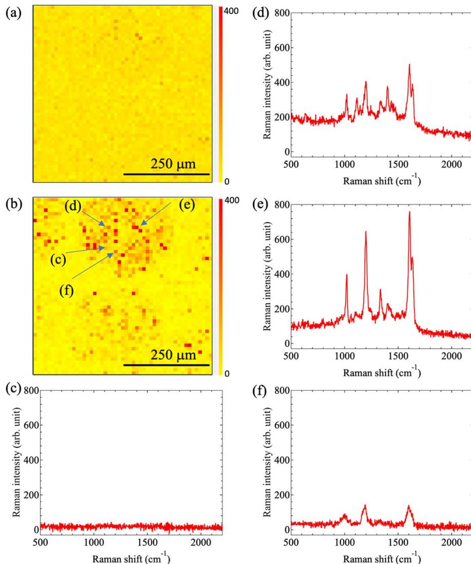
Fig. 15 Raman intensity mapping images obtained at Raman shifts of (a) 2000 cm<sup>-1</sup> and (b) 1600 cm<sup>-1</sup> in the case of printing using ink 'C'. The observation area size of these two mapping images is 500 μm × 500 μm, with measurements being taken at a step size of 10 μm. (c)–(f) SERS spectra for the locations in the Raman mapping image shown in (b).
