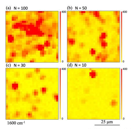
Fig. 4 Raman intensity mapping images obtained in cases where the shot number N is (a) 100, (b) 50, (c) 30, and (d) 10, when printing using ink 'A'. Here, the observation area was set at 50  $\mu$ m  $\times$  50  $\mu$ m with measurements being taken using a step size of 2.5  $\mu$ m. Raman mapping images acquired at 1600 cm<sup>-1</sup> are shown. The red (yellow) color denotes the high (low) Raman intensity.
