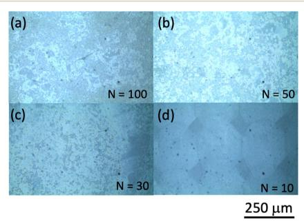
Fig. 2 Optical microphotographs of areas printed using ink 'A' with number of shots N of (a) 100, (b) 50, (c) 30, and (d) 10. The scale bar length is 250 μm.
