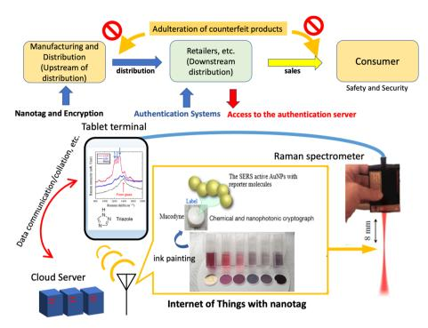
Fig. 1 Schematic of authentication systems based on nanotags for logistics from manufacturing to distribution, retailers, sales, resales, and the consumer, providing safety and security.
