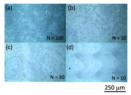
Fig. 5 Optical microphotographs of printed areas using ink 'B' with number of shots N of (a) 100, (b) 50, (c) 30, and (d) 10. The scale bar length is 250  $\mu$ m.
