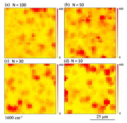
Fig. 6 Raman intensity mapping images obtained in cases where the shot number N is (a) 100, (b) 50, (c) 30, and (d) 10, when printing using ink 'B'. Here, the observation area was set at 50  $\mu$ m  $\times$  50  $\mu$ m with measurements being taken at a step size of 2.5  $\mu$ m. Raman mapping images acquired at 1600 cm<sup>-1</sup> are shown. The red (yellow) color indicates the high (low) Raman intensity.
