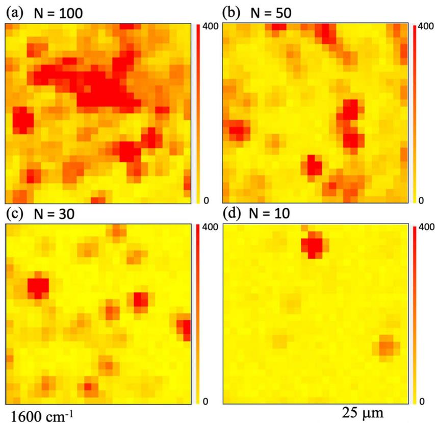
Fig. 4 Raman intensity mapping images obtained in cases where the shot number  $N$  is (a) 100, (b) 50, (c) 30, and (d) 10, when printing using ink 'A'. Here, the observation area was set at  $50\ \mu\text{m} \times 50\ \mu\text{m}$  with measurements being taken using a step size of  $2.5\ \mu\text{m}$ . Raman mapping images acquired at  $1600\ \text{cm}^{-1}$  are shown. The red (yellow) color denotes the high (low) Raman intensity.
