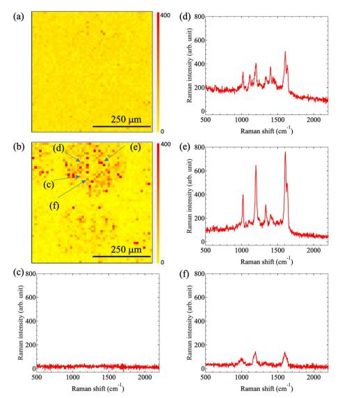
Fig. 15 Raman intensity mapping images obtained at Raman shifts of (a) 2000 cm $^{-1}$  and (b) 1600 cm $^{-1}$  in the case of printing using ink 'C'. The observation area size of these two mapping images is 500  $\mu$ m  $\times$  500  $\mu$ m, with measurements being taken at a step size of 10  $\mu$ m. (c)–(f) SERS spectra for the locations in the Raman mapping image shown in (b).
