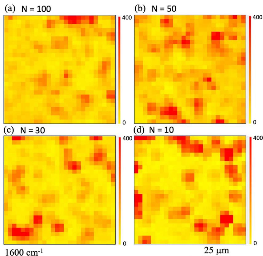
Fig. 6 Raman intensity mapping images obtained in cases where the shot number  $N$  is (a) 100, (b) 50, (c) 30, and (d) 10, when printing using ink 'B'. Here, the observation area was set at  $50 \mu\text{m} \times 50 \mu\text{m}$  with measurements being taken at a step size of  $2.5 \mu\text{m}$ . Raman mapping images acquired at  $1600 \text{ cm}^{-1}$  are shown. The red (yellow) color indicates the high (low) Raman intensity.
