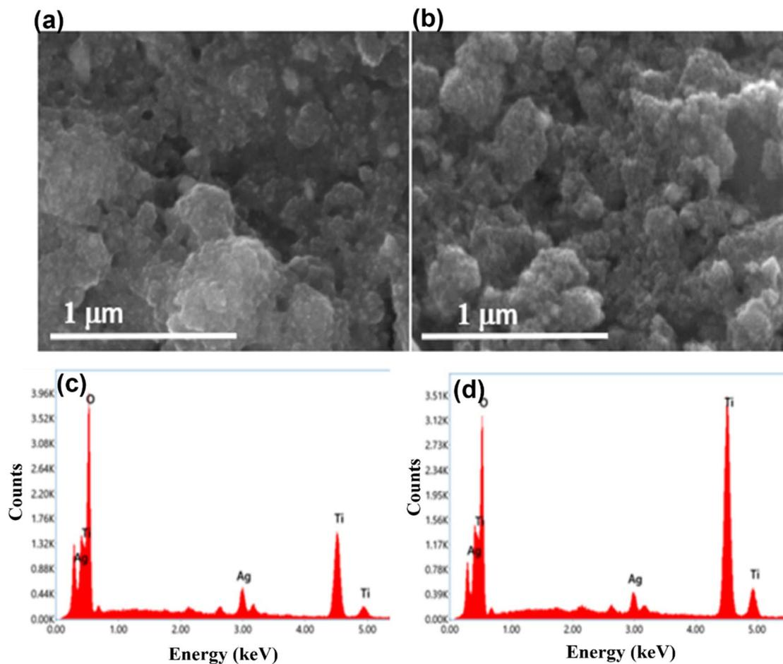
Fig. 6 (a and b) SEM images and (c and d) EDAX spectra of green-synthesized Ag-TiO<sub>2</sub> NCs (*A. indica* and *M. indica*).
