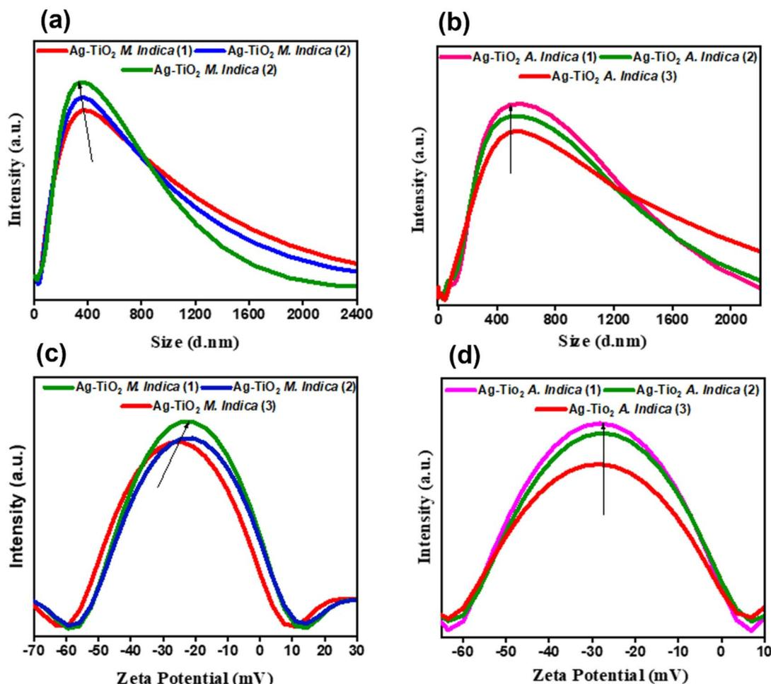
Fig. 4 (a and b) Dynamic light scattering and Z-average hydrodynamic diameter of Ag-TiO<sub>2</sub> NCs (*A. indica* and *M. indica*), (c and d) zeta potential measurements for Ag-TiO<sub>2</sub> NCs synthesized using *A. indica* and *M. indica* leaf extracts.
