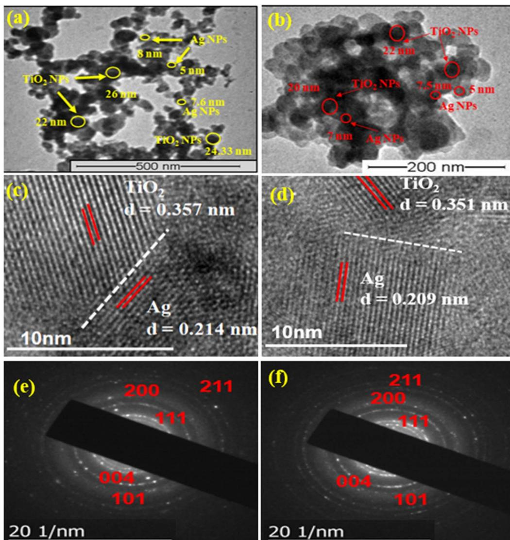
Fig. 5 (a and b) TEM images (c and d) HRTEM images (e and f) SAED images of Ag-TiO<sub>2</sub> NCs synthesized using *A. indica* and *M. indica* leaf extracts.
