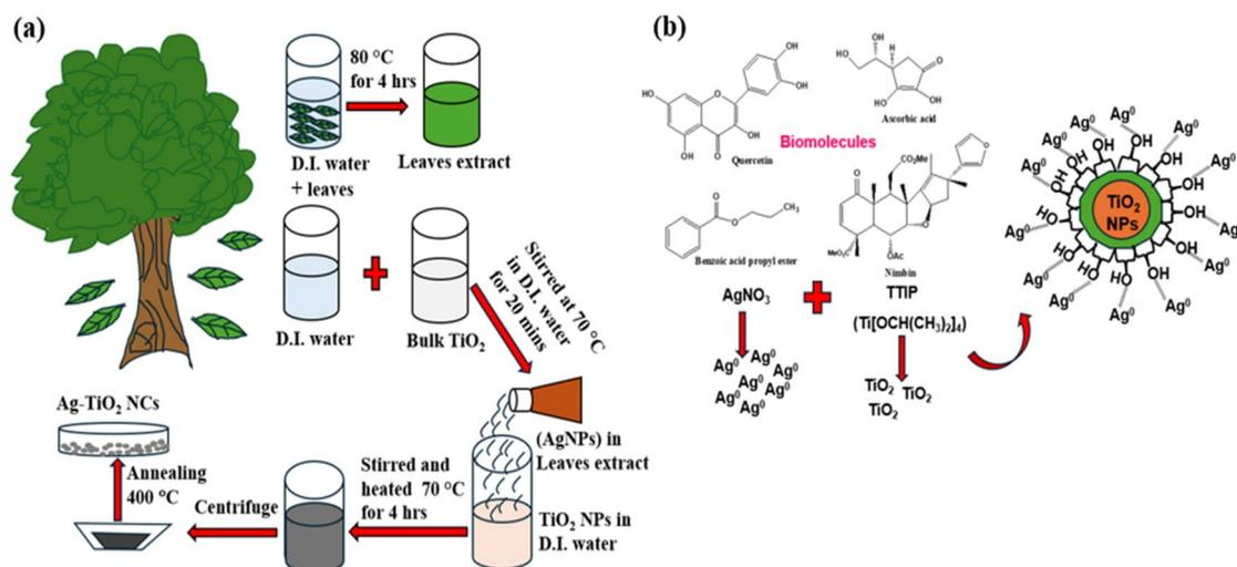
Fig. 1 Schematic of (a) the proposed green synthesis route of Ag–TiO<sub>2</sub> NCs using *A. indica* and *M. indica* leaf extracts and (b) mechanism of Ag–TiO<sub>2</sub> NCs.
