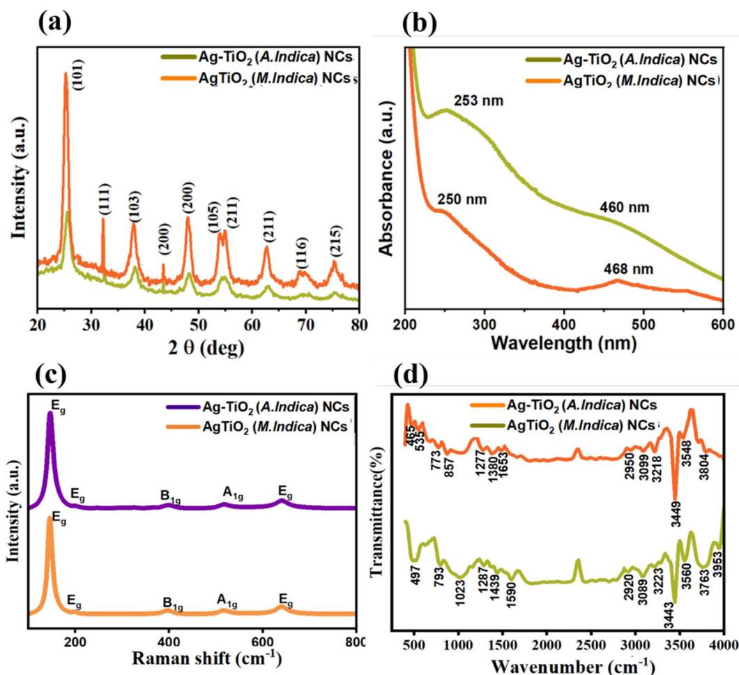
Fig. 3 (a) X-ray diffraction (XRD) patterns of Ag-TiO<sub>2</sub> NCs and (b) UV-vis spectra of Ag-TiO<sub>2</sub> NCs synthesized using *A. indica* and *M. indica* leaf extracts, (c) Raman spectra of Ag-TiO<sub>2</sub> NCs and (d) FTIR spectra of Ag-TiO<sub>2</sub> NCs synthesized using leaf extracts of *A. indica* and *M. indica*.
