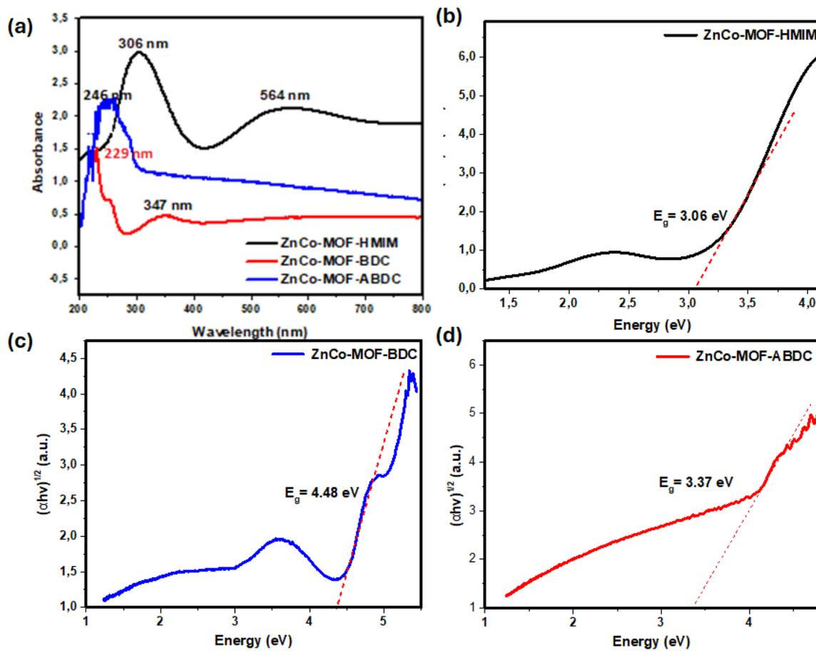
Fig. 9 (a) UV-visible spectra and (b–d) band gap plots of ligand-modified Zn Co MOFs.
