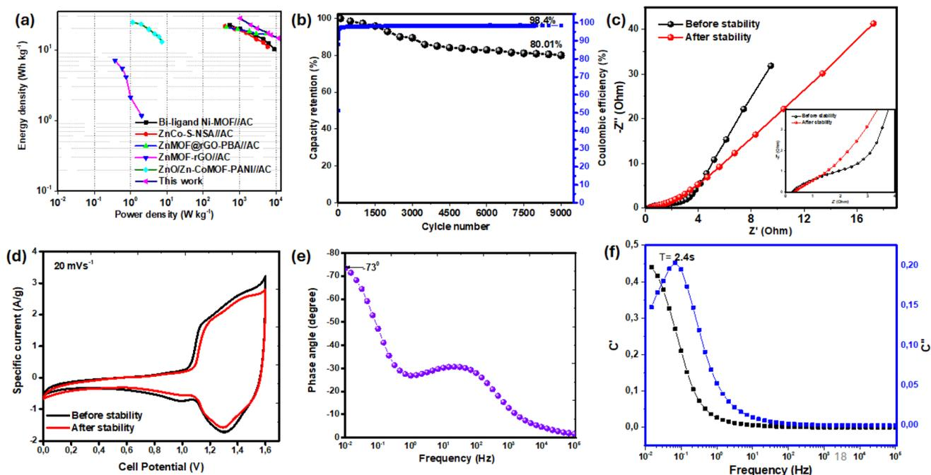
Fig. 14 (a) Ragone plot of the device, (b) cycling stability test after 10 000 cycles at  $10 \text{ A g}^{-1}$ , (c) Nyquist plot with an inset showing high frequency zone magnification before and after cycle stability, (d) CV plots before and after stability, (e) Bode plot and (f) imaginary and real capacitance vs. frequency of the hybrid device.
