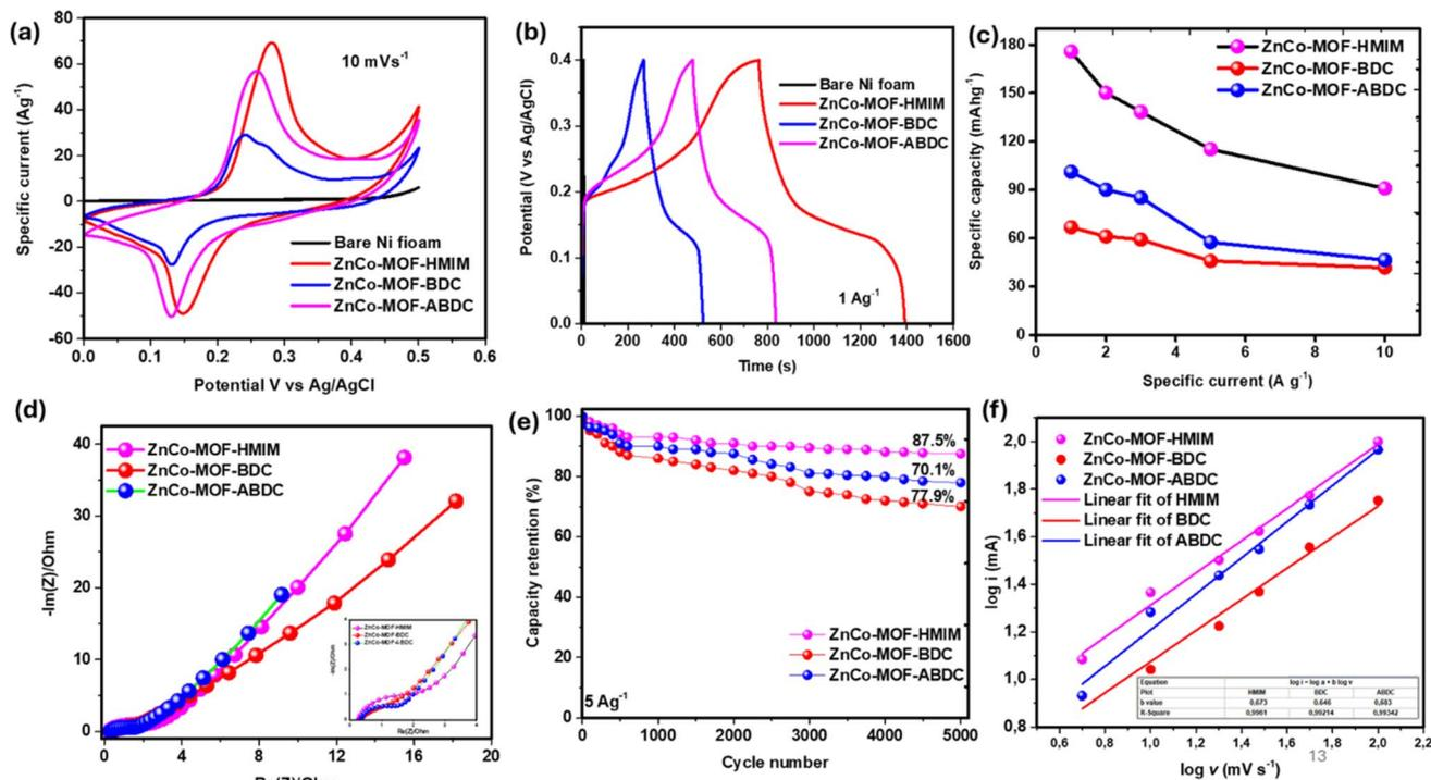
Fig. 10 (a) CV curves of ZnCo-MOFs at 10 mV s<sup>-1</sup>, (b) GCD curves of ZnCo-MOFs at 1 A g<sup>-1</sup>, (c) the specific capacity at various specific currents, (d) Nyquist plots and (e) cycling stability at 5000 cycles of ZnCo-MOFs at 10 A g<sup>-1</sup> (f) plot of log of the current vs. scan rate.
