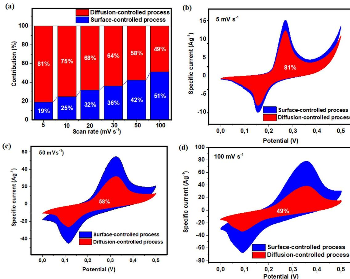
Fig. 12 (a) Contributions of charge storage mechanisms against scan rate, CV curves with displaying contributions of each process at (b) 5 mV s<sup>-1</sup>, (c) 50 mV s<sup>-1</sup> and (d) 100 mV s<sup>-1</sup> of ZnCo-MOF-HMIM.
