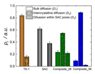
Fig. 7 Pre-exponential factor  $p_i$  component of eqn (1) in the diffusion of MO for TS-1, SAC, Composite\_26, and Composite\_56.
