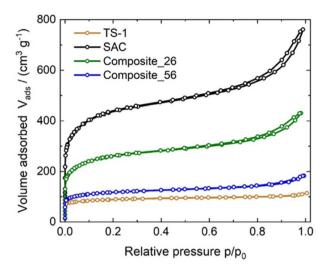
Fig. 1 Nitrogen sorption isotherms displayed as volume adsorbed ( $V_{\rm ads}$ ) over relative pressure ( $p/p_0$ ) of TS-1, SAC, Composite\_26 and Composite\_56 recorded at 77 K.
