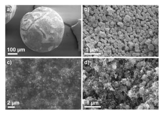
Fig. 3 SEM images showing the exterior of a single TS-1/SAC Composite\_26 particle (a) and a close-up view of TS-1 crystallites occupying the surface (b). BSE-SEM (c) and SEM detail image (d) of a cross-section of a split spherical particle showing the presence of TS-1 crystallites.
