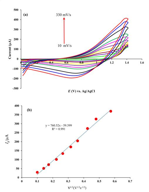
Fig. 6 (a) CVs of 10 nM VGCV in 0.1 M phosphate buffer solution (pH = 7.4) at different scan rates of 10, 20, 30, 50, 70, 100, 130, 180, 230 and 330 mV s<sup>-1</sup>; (b) corresponding plot of oxidation peak current vs. square root of potential scan rate.
