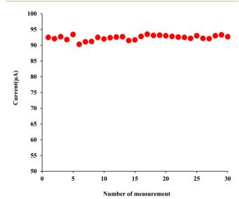
Fig. 9 Response of the designed sensor to a solution of valganciclovir with 600 nM concentration in 30 consecutive measurements at pH = 7 and a scan rate of 100 mV s<sup>-1</sup>.
