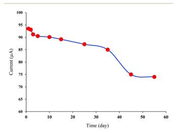
Fig. 8 Sensor response  $(I_p)$  to a solution of valganciclovir with 600 nM concentration over a period of 55 days after fabrication and storage at room temperature at pH = 7 and a scan rate of 100 mV s<sup>-1</sup>.
