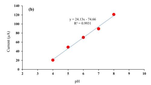
Fig. 5 (a) Influence of pH on the peak current ( $I_p$ ) for a solution with 0.75  $\mu$ M VGCV in phosphate buffer; (b) the linear range between pH 4 and 8.
