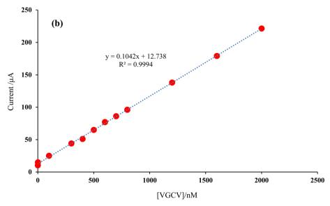
Fig. 7 (a) DPVs of different concentrations of VGCV from 0.1 to 2000 nM in 0.1 M phosphate buffer solution (pH = 7.4); (b) resulted standard calibration curve. Error bars obtained for three trials.
