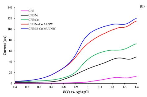
Fig. 3 (a) Cyclic voltammograms of VGCV recorded at the surface of different fabricated electrodes; (b) comparison DPV response of CPE, CPE/Ni, CPE/Co, Co-Ni(ALNW)/CPE and Co-Ni(MLNW)/CPE electrodes. The concentration of VGCV is 900 nM in PBS 0.1 M (pH 7.4) at a scan rate of 100 mV s<sup>-1</sup>.
