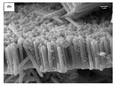
Fig. 1 SEM images of (a) Co-Ni multilayer nanowires; (b) Co-Ni alloy nanowires prepared in the AAO template and released from template by dissolving the template in NaOH.
