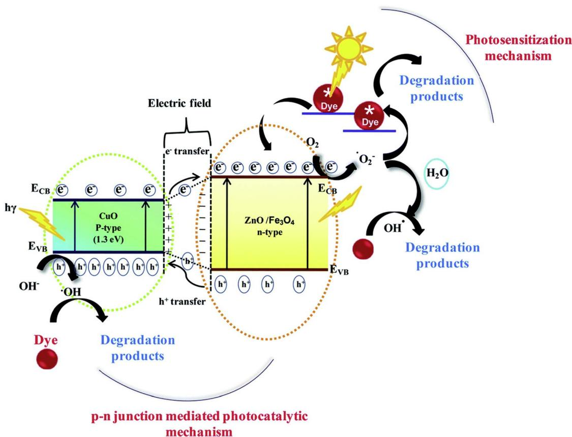
Fig. 8 Photocatalytic degradation pathway under the solar light irradiation using the p–n heterojunctions (ZnO–CuO or Fe<sub>3</sub>O<sub>4</sub>–CuO).<sup>127</sup> Copyright 2016 Elsevier.
