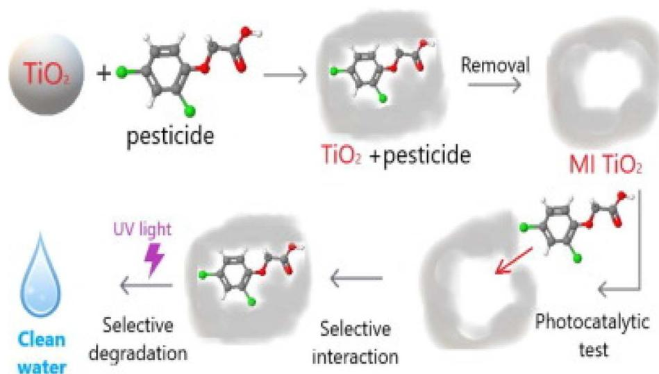
Fig. 5 Preferential removal of pesticides from water by molecular imprinting on TiO<sub>2</sub> photocatalysts.<sup>73</sup>
