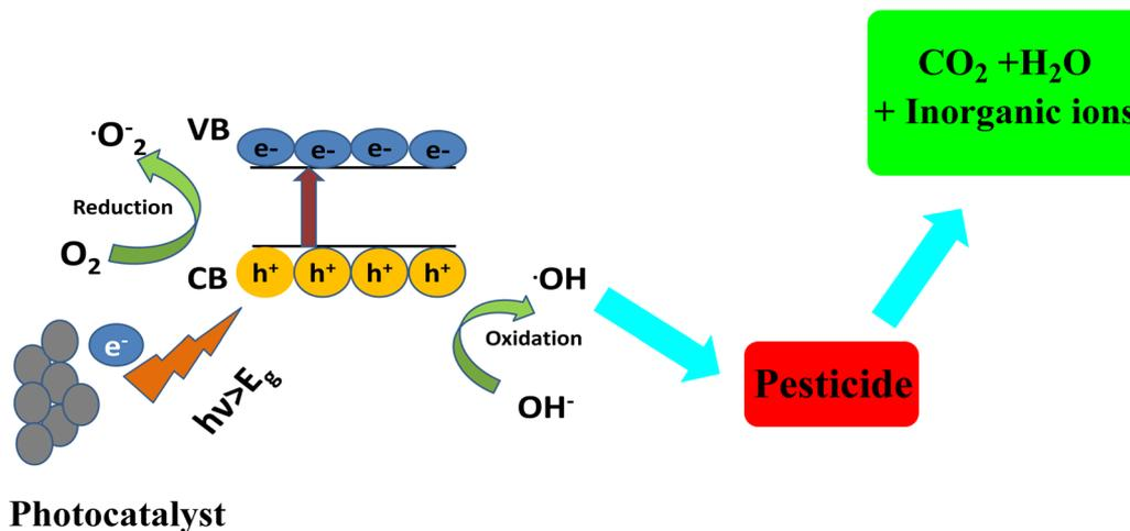
Fig. 3 Photocatalytic degradation of pesticides using photocatalysts.
