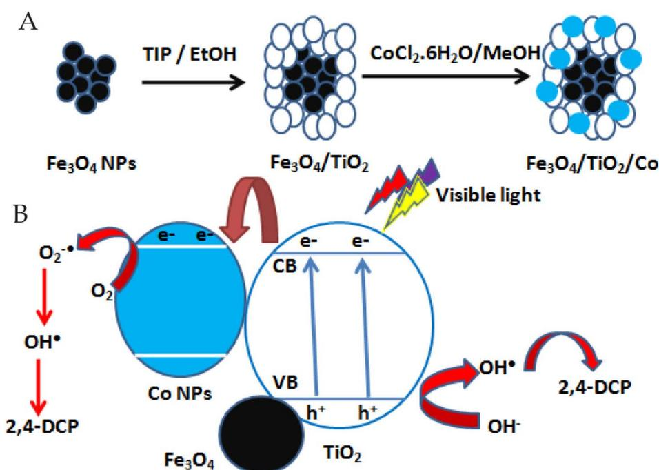
Fig. 4 2,4-Dichlorophenol degradation via photo-reactive  $\text{TiO}_2$  nanoparticles, (A) preparation of the photocatalyst; (B) the degradation pathway of 2,4-DCP.<sup>69</sup>
