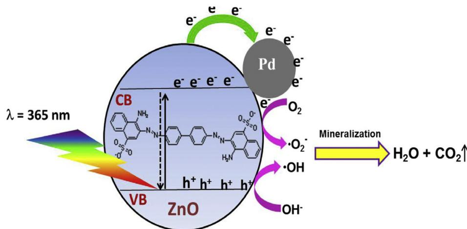
Fig. 6 Schematic diagram illustrating the plausible photocatalytic mechanism for degradation of Congo red dye using the Pd-doped ZnO photocatalyst.<sup>93</sup> Reprinted with permission from Copyright 2016 Elsevier.
