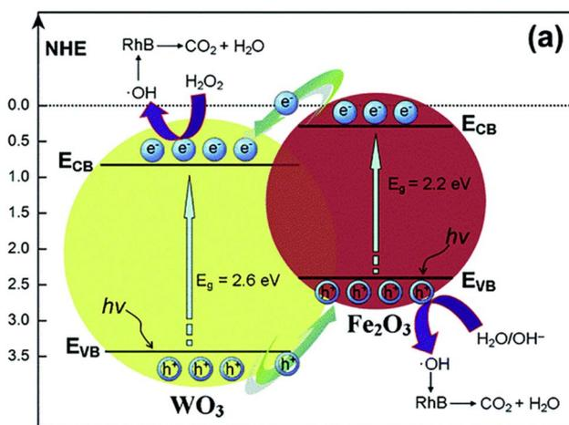
Fig. 9 Mechanism pathway of light-induced charge separation in the Fe<sub>2</sub>O<sub>3</sub>–WO<sub>3</sub> nanocomposite and photo-degradation of Rhodamine B.<sup>132</sup> Copyright 2014 Royal Society of Chemistry.
