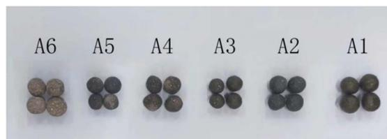
Fig. 5 Photos of sintered ceramsites made from CG, FA and SS with different proportions.
