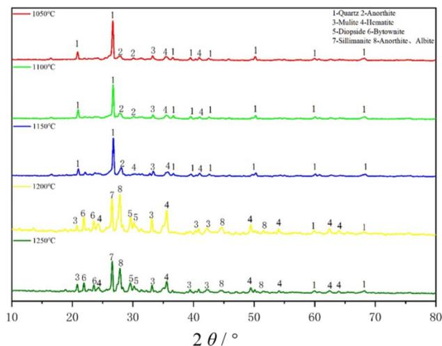
Fig. 14 XRD of samples at different temperatures.
