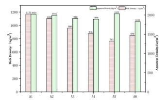
Fig. 7 Bulk density and apparent density of ceramsites produced from different mixtures.
