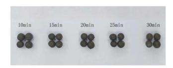
Fig. 15 Morphology of ceramsite at different sintering time.
