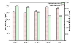
Fig. 11 Bulk density and apparent density of ceramsite at different sintering temperatures.
