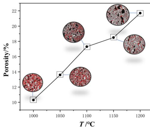
Fig. 13 Porosity of ceramsite at different sintering temperatures.
