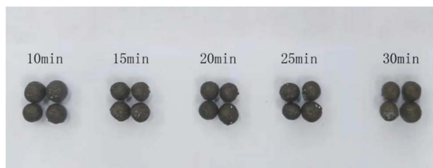
Fig. 15 Morphology of ceramsite at different sintering time.
