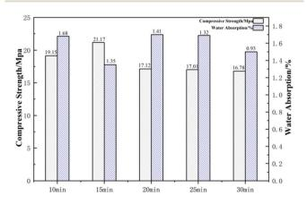
Fig. 16 Strength and water absorption of ceramsite at different sintering time.
