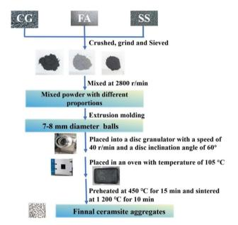
Fig. 4 Production process of ceramsite aggregates
