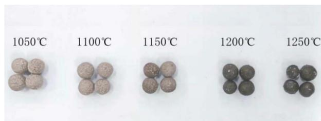
Fig. 12 Morphology of ceramsite at different sintering temperatures.
