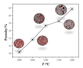
Fig. 13 Porosity of ceramsite at different sintering temperatures.
