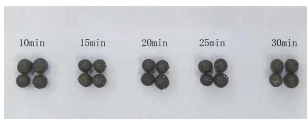
Fig. 15 Morphology of ceramsite at different sintering time.
