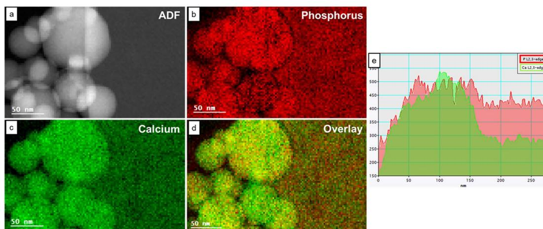
Fig. 4 (a) The STEM Annular Dark Field (ADF) image and the corresponding EELS elemental mapping of (b) the P  $L_{2,3}$ -edge and (c) the Ca  $L_{2,3}$ -edge. (d) The overlay of phosphorus map and calcium map. The red color represents the phosphorus signal, and the green color represents the calcium signal. (e) The intensity projection of P and Ca signal to the *x*-axis. The *x*-axis represents the distance from left to right, and the *y*-axis indicates the intensities of P and Ca.
