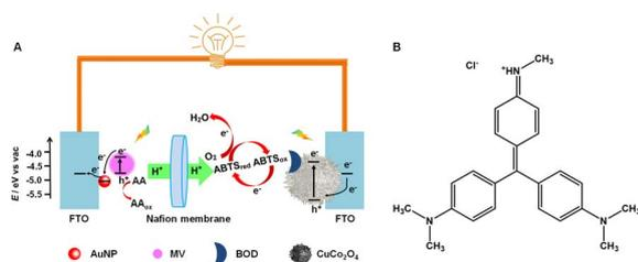
**Scheme 2** (A) Schematic drawing of the working principle of a PEBFC equipped with a (MV/AuNPs)<sub>25</sub>/FTO photoanode, a BOD/ $\text{CuCo}_2\text{O}_4$ /FTO bio-photocathode and a Nafion membrane. (B) The structural formula of MV, [4-[[4-(dimethylamino)phenyl]-[4-(methylamino)phenyl]methylidene]cyclohexa-2,5-dien-1-ylidene]-dimethylazanium chloride.
