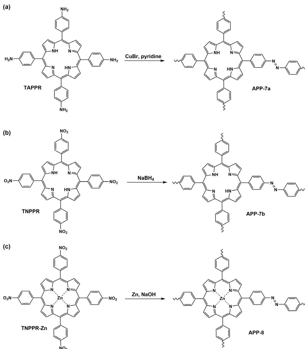
Fig. 2 Synthesis of **APP-7a**, **APP-7b** and **APP-8** by homocoupling methods. (a) Cu(I)-catalysed oxidative homocoupling of **TAPPR**, (b) NaBH<sub>4</sub>-mediated reductive homocoupling of **TNPPR** and (c) Zn-induced reductive homocoupling of **TNPPR-Zn**.
