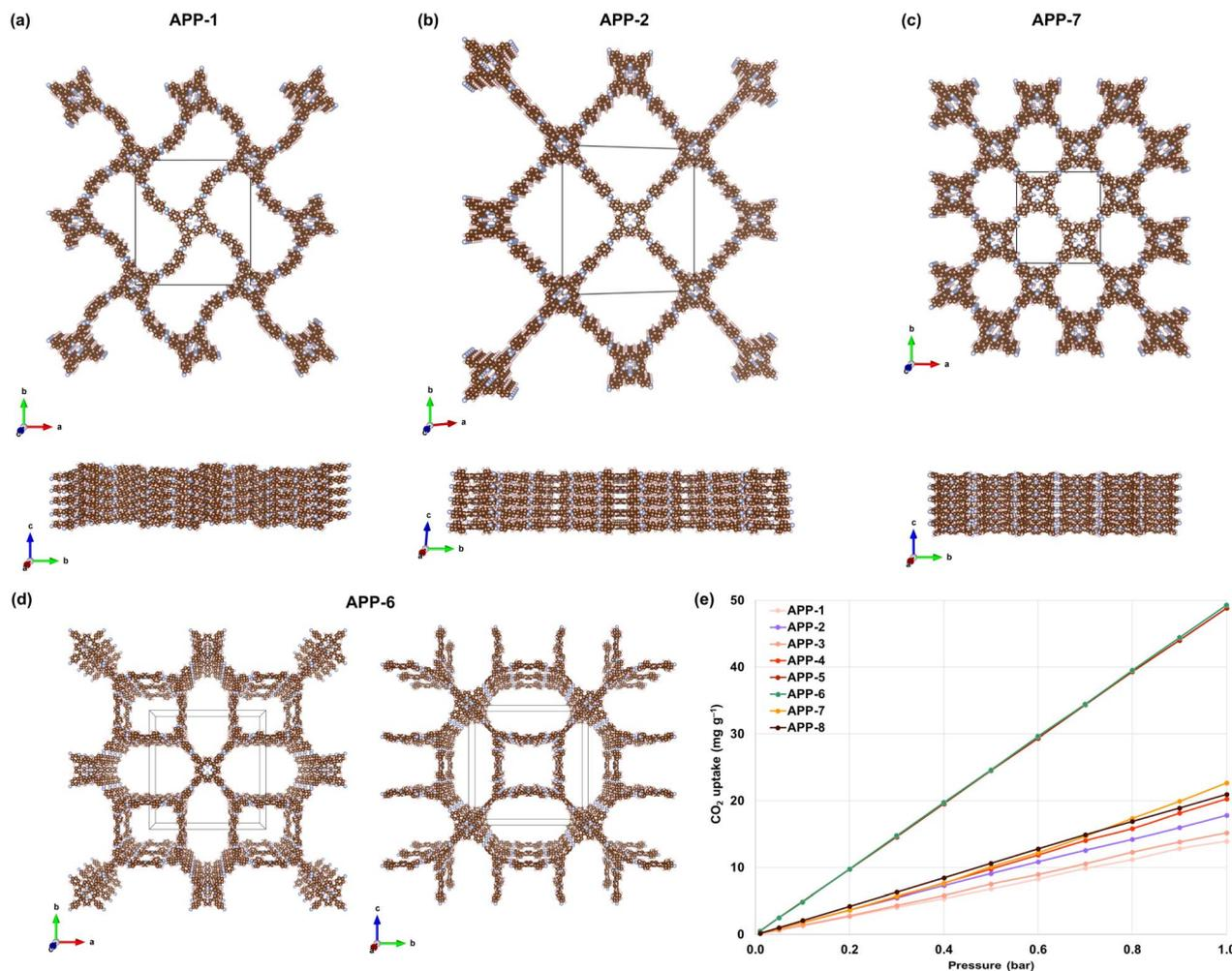
Fig. 7 Optimized geometries (PBE-D3/pob-TZVP-rev2) of: (a) 2D-layered APP-1, (b) 2D-layered APP-2, (c) 2D-layered APP-7 and (d) 3D APP-6. Views along the crystallographic *a* and *c* axes. (e) CO<sub>2</sub> adsorption isotherms of modeled APPs at 298 K.
