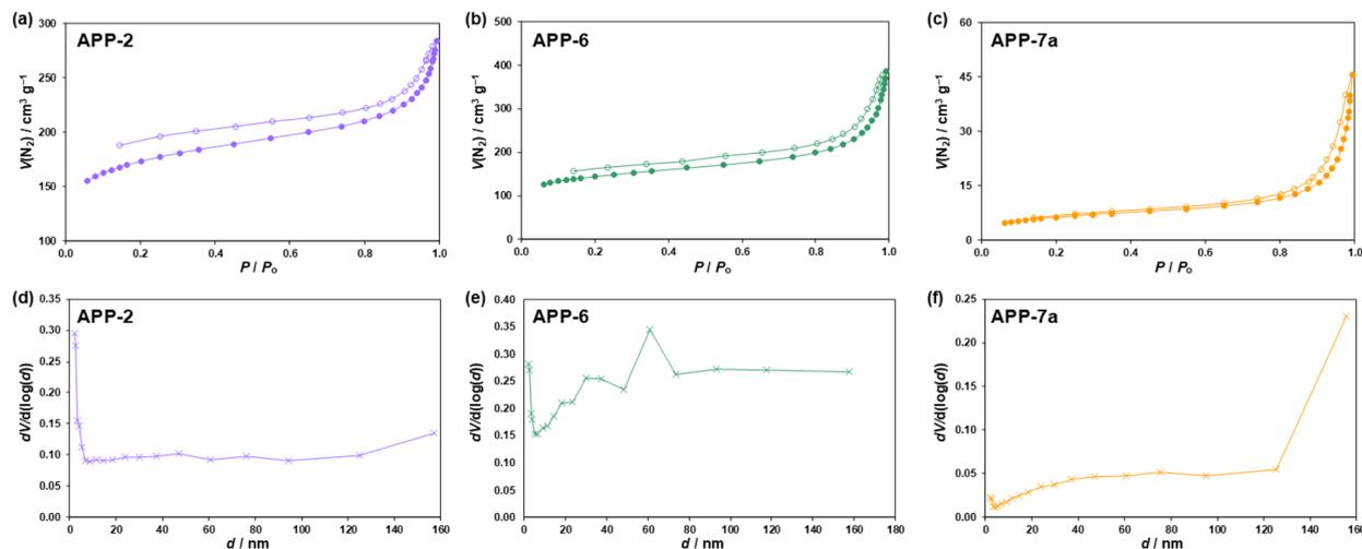
Fig. 5 Representative N<sub>2</sub> adsorption–desorption isotherms of: (a) APP-2, (b) APP-6 and (c) APP-7a measured at 77 K. The adsorption and desorption isotherms are depicted with filled and open markers, respectively. Pore size distributions of: (d) APP-2, (e) APP-6 and (f) APP-7a.
