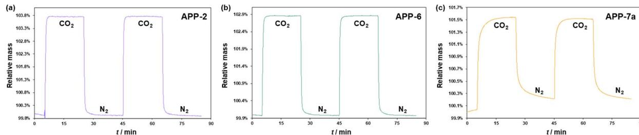
Fig. 6 Representative thermogravimetric CO<sub>2</sub> adsorption and desorption profiles of (a) APP-2, (b) APP-6 and (c) APP-7a at approximately 306 K.
