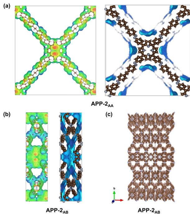
Fig. 8 Electrostatic potential maps (left panel) and density plots (right panel) showing the average CO<sub>2</sub> distribution at 298 K and 1 bar for AA stacking (a) and AB stacking (b) modes of APP-2. Optimized geometry (PBE-D3/pob-TZVP-rev2) of AB stacked APP-2 (c).
