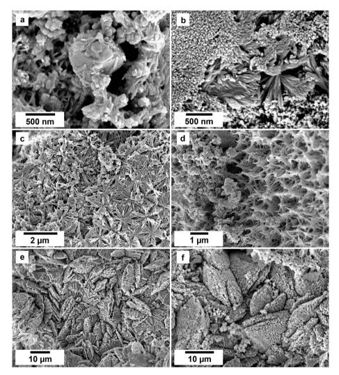
Fig. 5 SEM photomicrographs showing the nanocrystals obtained in the experiments at 165 °C in the PAAS solution experiments. (a) Surface of ginite becoming covered by rhabdophane nanorods; (b and c) growth of rhabdophane nanocrystals on the surface of the host, sometimes forming spherulitic-type aggregates (c); (d) nanocrystals of hematite on rhabdophane. (e and f) Monazite and rhabdophane aggregates.
