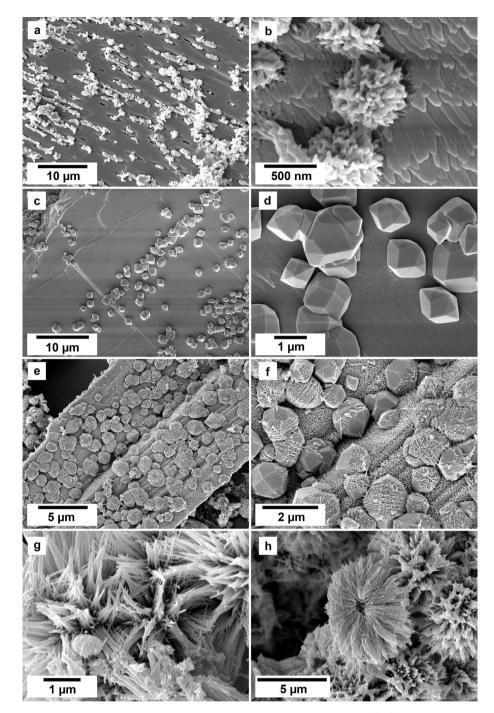
Fig. 4 SEM photomicrographs showing the nanocrystalline solids obtained in the experiments at 90 °C using equal REE concentration solutions. (a and b) Surface of vivianite becoming covered by metavivianite nanoaggregates; (c and d) growth of giniite crystals on the surface of the vivianite; (e and f) early stages of growth of rhabdophane on the surface of giniite. (g and h) Rhabdophane nanoaggregates and spherulites covering the surface of the host crystals.
