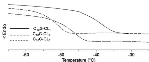
Fig. 9 DSC thermograms [glass transition temperature ( $T_g$ )] for species derived from monodisperse oligo(CL) from geraniol: monomer ( $\text{C}_{15}\text{G-CL}_1$ ), dimer ( $\text{C}_{15}\text{G-CL}_2$ ) and trimer ( $\text{C}_{15}\text{G-CL}_3$ ).
