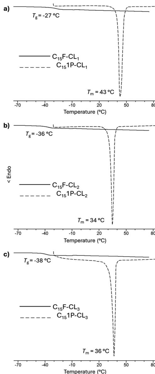
Fig. 10 DSC thermograms for species derived from farnesol ( $\text{C}_{15}\text{F-CL}_x$ ) and 1-pentadecanol ( $\text{C}_{15}\text{1P-CL}_x$ ) (where  $x = 1, 2, 3$ ): (a) monomer, (b) dimer and (c) trimer.
