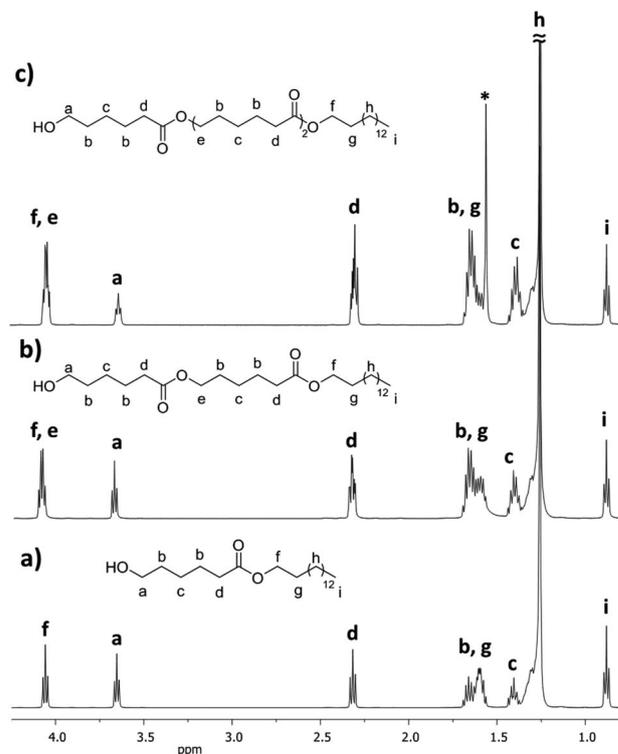
Fig. 7  $^1H$  NMR (500 MHz) spectra in  $CDCl_3$  of the monodisperse oligomers derived from  $\epsilon$ -caprolactone (CL) functionalized with 1-pentadecanol, isolated by flash column chromatography (FCC), (a) monomer  $C_{15}P-CL_1$ , (b) dimer  $C_{15}P-CL_2$ , and (c) trimer  $C_{15}P-CL_3$  (Table 2) (\* signal of the water).
