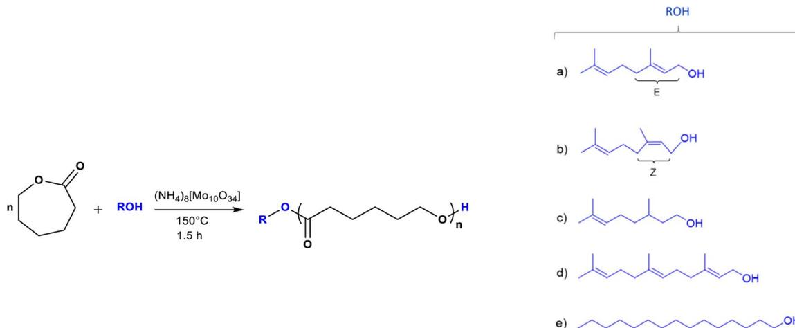
**Scheme 1** Synthesis of oligo( $\epsilon$ -caprolactones) [oligo(CLs)] catalyzed by ammonium decamolybdate  $[(\text{NH}_4)_8(\text{Mo}_{10}\text{O}_{34})]$  using different types of initiators (R-OH): (a) geraniol ( $\text{C}_{10}$ ), (b) nerol ( $\text{C}_{10}$ ), (c)  $\beta$ -citronellol ( $\text{C}_{10}$ ), (d) farnesol ( $\text{C}_{15}$ ), and (e) 1-pentadecanol ( $\text{C}_{15}$ ).
