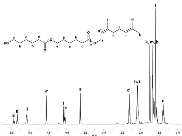
**Fig. 1** <sup>1</sup>H NMR (500 MHz) spectrum of oligo(CL) synthesized using nerol as initiator (C<sub>10</sub>N-PCL, Table 1) in CDCl<sub>3</sub> at 40 °C. Signal f [methylene, HO-CH<sub>2</sub>-CH=C] and g [methine, HO-CH<sub>2</sub>-CH=C] are from unreacted nerol.
