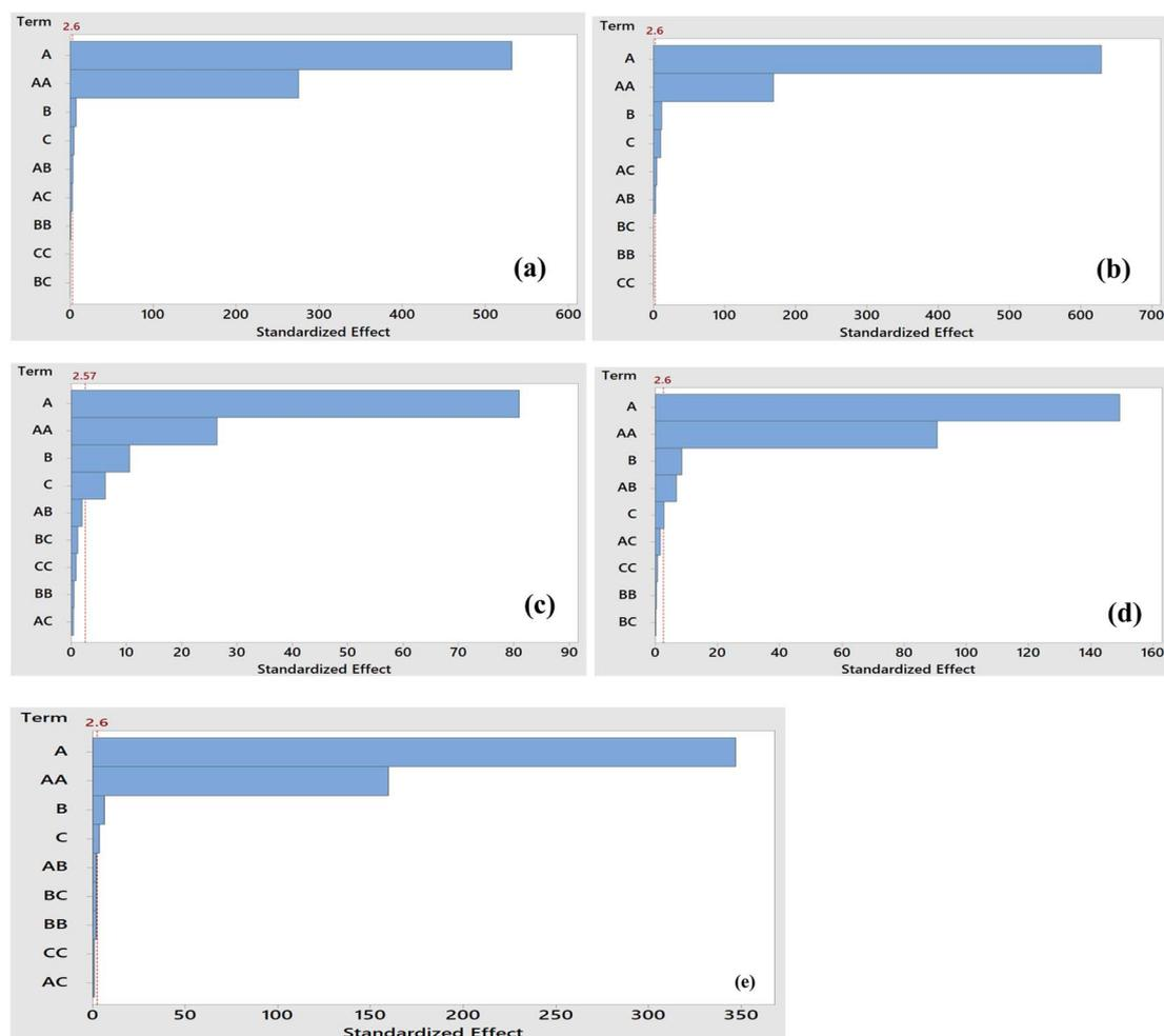
Fig. 3 Pareto charts of standardized effects for residual  $\text{Cr}(\text{VI})$  concentration ( $\text{mg L}^{-1}$ ) by the reagent (a)  $\text{FeSO}_4$ , (b)  $\text{Na}_2\text{S}$ , (c)  $\text{Na}_2\text{S}_2\text{O}_3$ , (d)  $\text{Na}_2\text{S}_2\text{O}_5$ , (e)  $\text{Na}_2\text{SO}_3$ .
