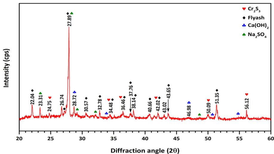
Fig. 7 XRD patterns of stabilized Cr contaminated soil sample with sodium thiosulphate as stabilizing reagent. The different symbols were used to depict the presence of  $\text{Cr}_2\text{S}_3$ , fly ash,  $\text{Ca}(\text{OH})_2$  and  $\text{Na}_2\text{SO}_4$  diffraction peaks.
