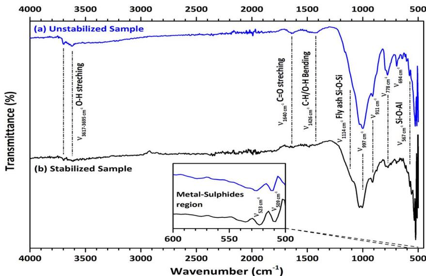
Fig. 6 FTIR spectrum of chromium contaminated sample before and after stabilization.
