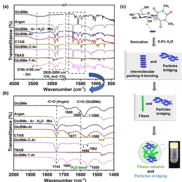
Fig. 2 (a) IR spectra (4000–450 cm<sup>-1</sup>) and (b) (2000–1400 cm<sup>-1</sup>) of **GlcBMe**, argan oil, **GlcBMe**-Ar-H<sub>2</sub>O-mix, **GlcBMe**-Ar, CTAB, **GlcBMe**-C-Ar, TBAB and **GlcBMe**-T-Ar (c) illustration of self-assembly mechanism.
