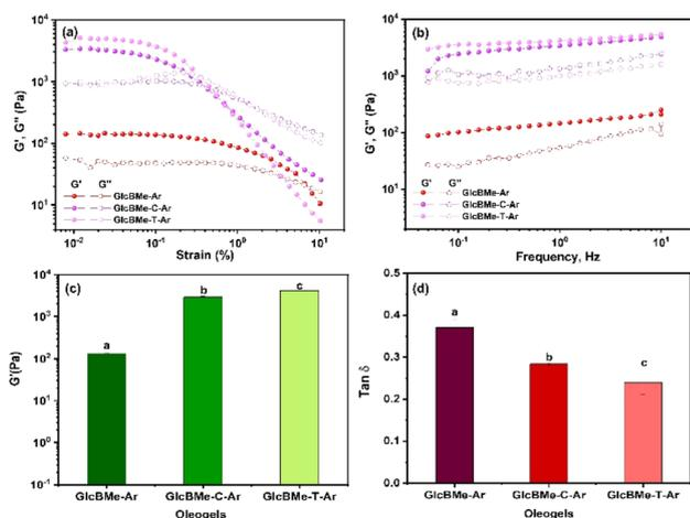
Fig. 4 Rheological behavior of oleogels (a) strain sweeps (b) frequency sweep (c)  $G'$  vs. oleogels (d)  $\tan \delta$  vs. oleogels for samples **GlcBMe–Ar**, **GlcBMe–C–Ar**, **GlcBMe–T–Ar**. Different letters assigned to each bar represent statistical differences between the values across all samples ( $p < 0.05$ ).
