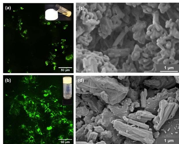
Fig. 1 CLSM microscopy images of (a) stained **GlcBMe** + Ar + H<sub>2</sub>O-mix before sonication then (b) stained **GlcBMe**-Ar oleogel; and SEM images of (c) as-prepared **GlcBMe** then (d) **GlcBMe** oleogelator obtained from oleogel washed out with acetone.
