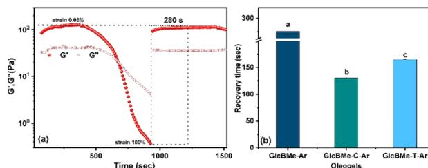
Fig. 5 (a) Thixotropic behavior for **GlcBMe–Ar** and (b) recovery time (s) in a two steps breakdown/buildup procedure for oleogel **GlcBMe–Ar**, **GlcBMe–C–Ar**, and **GlcBMe–T–Ar** \*statistically differences between the values across all samples ( $p < 0.05$ ). Different letters assigned to each bar represent statistical differences between the values across all samples ( $p < 0.05$ ).
