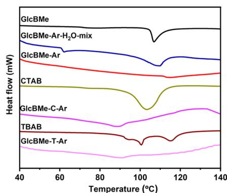
Fig. 3 DSC graph for **GlcBMe**, **GlcBMe**-Ar, **GlcBMe**-Ar + H<sub>2</sub>O-mix, **GlcBMe**-Ar, CTAB, **GlcBMe**-C-Ar, TBAB, **GlcBMe**-T-Ar. \*Analysis of **GlcBMe**, CTAB, and TBAB was made in oil.
