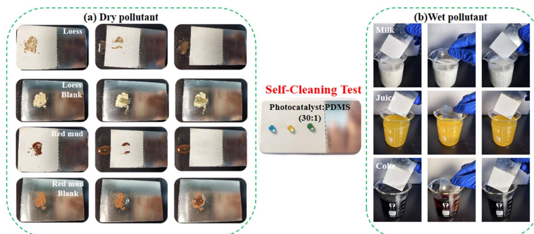
Fig. 11 Self-cleaning tests of photocatalytic superhydrophobic coatings on pollutants (mass ratio of photocatalytic material to PDMS 30 : 1) (a) dry pollutant; (b) wet pollutant.
