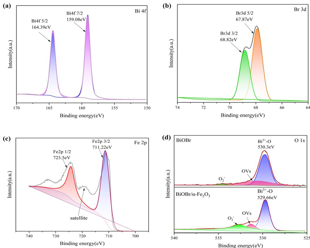
Fig. 4 XPS spectrum of BiOBr/ $\alpha$ -Fe<sub>2</sub>O<sub>3</sub> (a) Bi 4f; (b) Br 3d; (c) Fe 2p; (d) O 1s.
