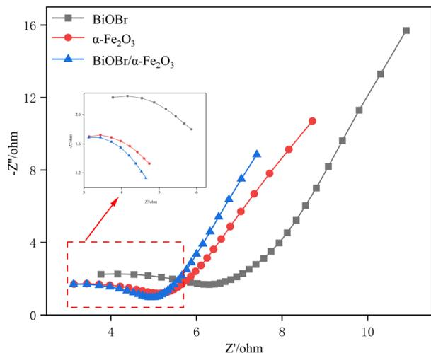
Fig. 6 Nyquist plots of BiOBr,  $\alpha$ -Fe<sub>2</sub>O<sub>3</sub> and BiOBr/ $\alpha$ -Fe<sub>2</sub>O<sub>3</sub>.
