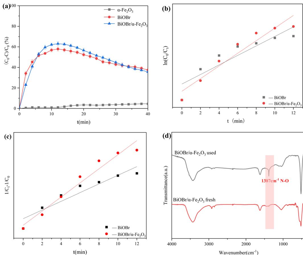
Fig. 7 (a) Degradation efficiency of NO by different photocatalytic materials; (b) primary kinetic analysis; (c) secondary kinetic analysis; (d) comparison of FTIR spectra of BiOBr/ $\alpha$ -Fe<sub>2</sub>O<sub>3</sub> before and after reaction.
