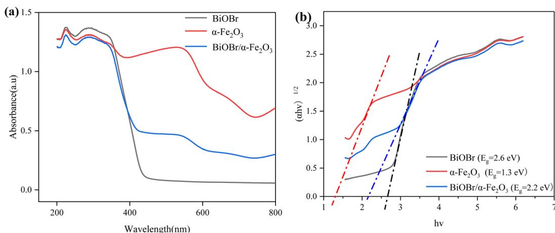
Fig. 5 (a) UV diffuse reflectance spectrum of BiOBr/ $\alpha$ -Fe<sub>2</sub>O<sub>3</sub>; (b) band gap spectrum of BiOBr/ $\alpha$ -Fe<sub>2</sub>O<sub>3</sub>.
