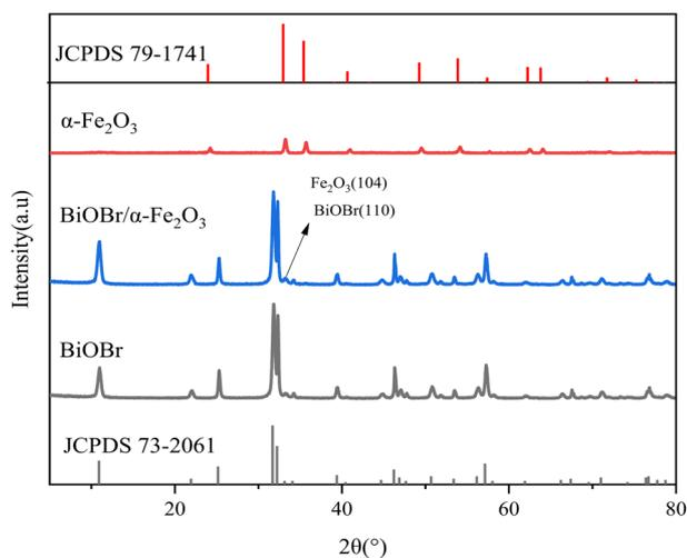
Fig. 3 XRD of BiOBr/ $\alpha$ - $\text{Fe}_2\text{O}_3$ .
