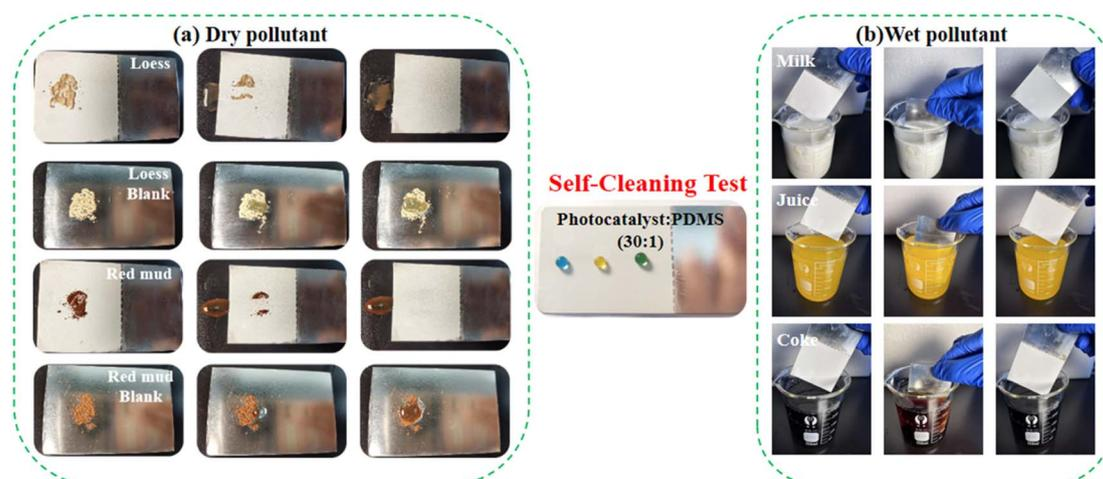
Fig. 11 Self-cleaning tests of photocatalytic superhydrophobic coatings on pollutants (mass ratio of photocatalytic material to PDMS 30 : 1) (a) dry pollutant; (b) wet pollutant.
