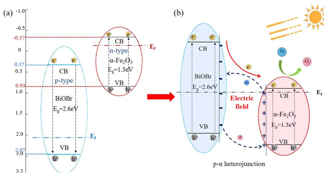
**Fig. 8** Heterogeneous structure building mechanism diagram for p-n type BiOBr/ $\alpha$ -Fe<sub>2</sub>O<sub>3</sub> photocatalysis. (a) Schematic electronic structures of BiOBr and  $\alpha$ -Fe<sub>2</sub>O<sub>3</sub>; (b) heterojunction mechanism diagram for p-n type BiOBr/ $\alpha$ -Fe<sub>2</sub>O<sub>3</sub> photocatalysis.
