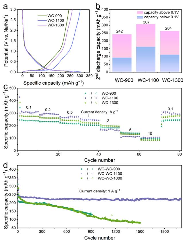
Fig. 3 (a) Galvanostatic discharge–charge profile of the 2nd cycle at  $0.1 \text{ A g}^{-1}$ , (b) the specific capacity contributions of the platform region  $<0.1 \text{ V}$  and the ramp region  $>0.1 \text{ V}$  are based on the discharge–charge curve of the second cycle, (c) rate performance, (d) cycling performance of the WC-900, WC-1100, and WC-1300 at  $1.0 \text{ A g}^{-1}$ .
