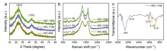
Fig. 2 (a) XRD and (b) Raman spectra of WC-900, WC-1100 and WC-1300 samples. (c) FTIR spectrum of the WC-1100
