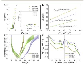
Fig. 4 (a) Nyquist plots, (b) Warburg value, (c) GITT profiles, and (d) Na<sup>+</sup> diffusion coefficients of the WC-900, WC-1100, and WC-1300, respectively.
