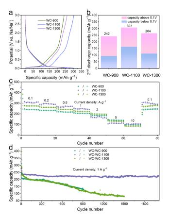
Fig. 3 (a) Galvanostatic discharge–charge profile of the 2nd cycle at 0.1 A g $^{-1}$ , (b) the specific capacity contributions of the platform region <0.1 V and the ramp region >0.1 V are based on the discharge–charge curve of the second cycle, (c) rate performance, (d) cycling performance of the WC-900, WC-1100, and WC-1300 at 1.0 A g $^{-1}$ .
