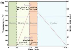
Fig. 1 Schematic diagram of TVS method for growing MoS<sub>2</sub> films.
