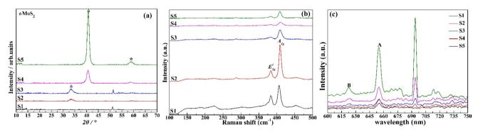
Fig. 4 Structural analysis of ex situ sulfurized Mo films (a) XRD spectra, (b) Raman spectra, (c) PL spectra
