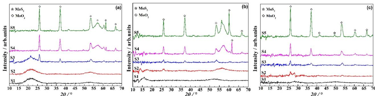
Fig. 2 The XRD spectra of *in situ* sulfurized Mo films under different carrier gas conditions, (a) 40 sccm of Ar and 10 of sccm H<sub>2</sub>; (b) 60 of sccm Ar and 10 of sccm H<sub>2</sub>; (c) 80 of sccm Ar and 20 of sccm H<sub>2</sub>.
