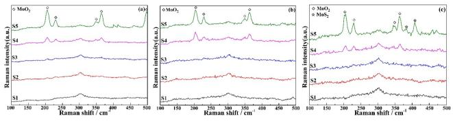
Fig. 3 The Raman spectra of in situ sulfurized Mo films under different carrier gas conditions, (a) 40 of sccm Ar and 10 of sccm H<sub>2</sub>; (b) 60 of sccm Ar and 10 of sccm H<sub>2</sub>; (c) 80 of sccm Ar and 20 of sccm H<sub>2</sub>.
