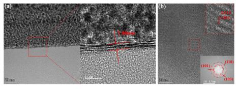
Fig. 6 (a) Cross-sectional TEM images and (b) crystalline structure of S1 sample.
