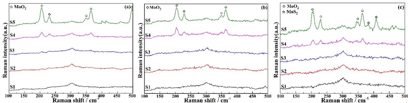
Fig. 3 The Raman spectra of *in situ* sulfurized Mo films under different carrier gas conditions, (a) 40 of sccm Ar and 10 of sccm H<sub>2</sub>; (b) 60 of sccm Ar and 10 of sccm H<sub>2</sub>; (c) 80 of sccm Ar and 20 of sccm H<sub>2</sub>.
