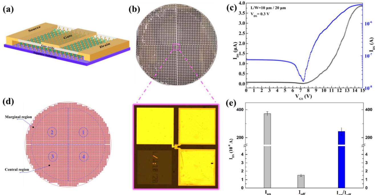
Fig. 7 (a) Schematic diagram of the top-gated MoS<sub>2</sub> TFT device; (b) the photographs of the TFT array devices integrated on a 2-inch sapphire wafer, and amplified optical microscope image of the single TFT device; (c) the typical transfer curves ( $I_{DS}$ – $V_{GS}$ ) of the trilayer MoS<sub>2</sub>-based TFT device; (d) schematic diagram of wafer device array; (e) statistical plot for the performances of 100 test devices.
