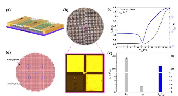
Fig. 7 (a) Schematic diagram of the top-gated  $MoS_2$  TFT device; (b) the photographs of the TFT array devices integrated on a 2-inch sapphire wafer, and amplified optical microscope image of the single TFT device; (c) the typical transfer curves ( $I_{DS}-V_{GS}$ ) of the trilayer  $MoS_2$ -based TFT device; (d) schematic diagram of wafer device array; (e) statistical plot for the performances of 100 test devices.
