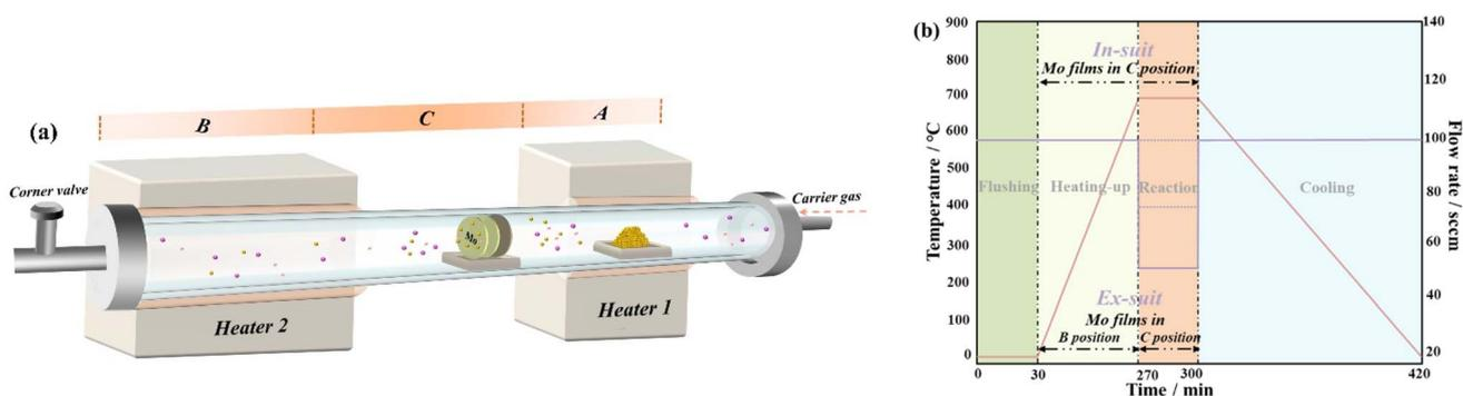
Fig. 1 Schematic diagram of TVS method for growing MoS<sub>2</sub> films.
