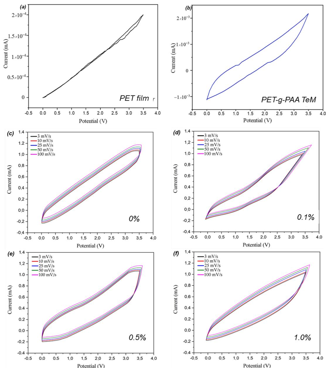
**Fig. 8** Cyclic voltammetry (CV) curves of pristine PET film (scan rate  $3 \text{ mV s}^{-1}$ ) (a), PAA-grafted TeM (scan rate  $3 \text{ mV s}^{-1}$ ) (b), and solid-state polymer supercapacitors based on varying GO content at different scan rates: 0% GO (c), 0.1% GO (d), 0.5% GO (e) 1% GO (f).
