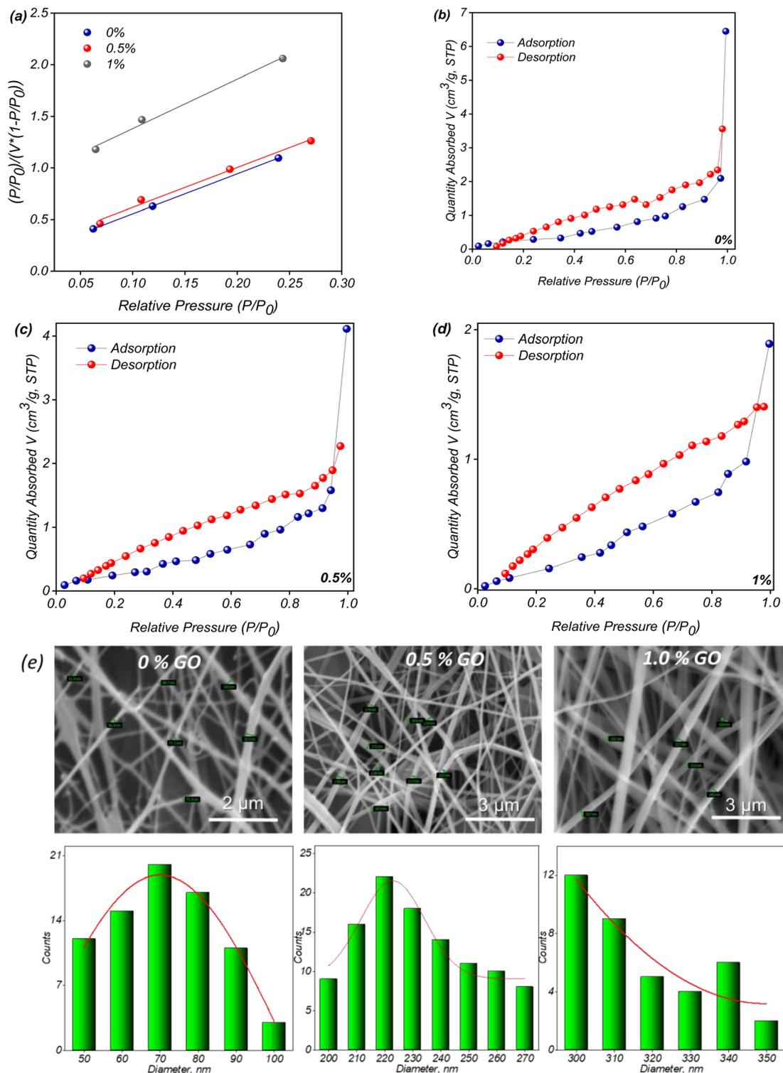
Fig. 7 BET-adsorption plot (a) and  $N_2$  adsorption-desorption isotherm of PVDF-HFP\_GO@PET-g-PAA membranes with different GO content of (b) 0%, (c) 0.5%, (d) 1%, the SEM images and corresponding size distributions composite nanofibers with different amount of GO (e).
