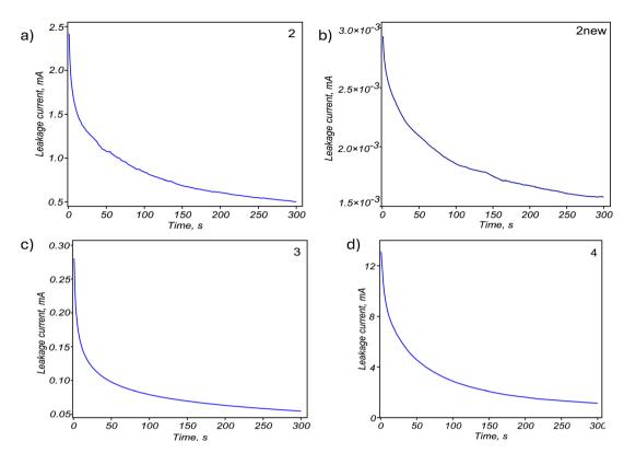
Fig. 14 Leakage current as a function of time for PVDF-HFP\_GO@PET-g-PAA solid-state supercapacitors with various GO content: 0% GO (a), 0.1% GO (b), 0.5% (c), 1% GO (d)
