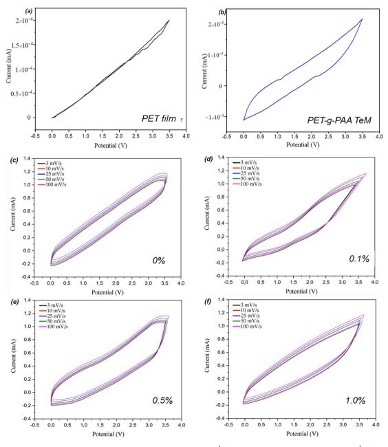
Fig. 8 Cyclic voltammetry (CV) curves of pristine PET film (scan rate 3 mV s $^{-1}$ ) (a), PAA-grafted TeM (scan rate 3 mV s $^{-1}$ ) (b), and solid-state polymer supercapacitors based on varying GO content at different scan rates: 0% GO (c), 0.1% GO (d), 0.5% GO, (e) 1% GO (f).
