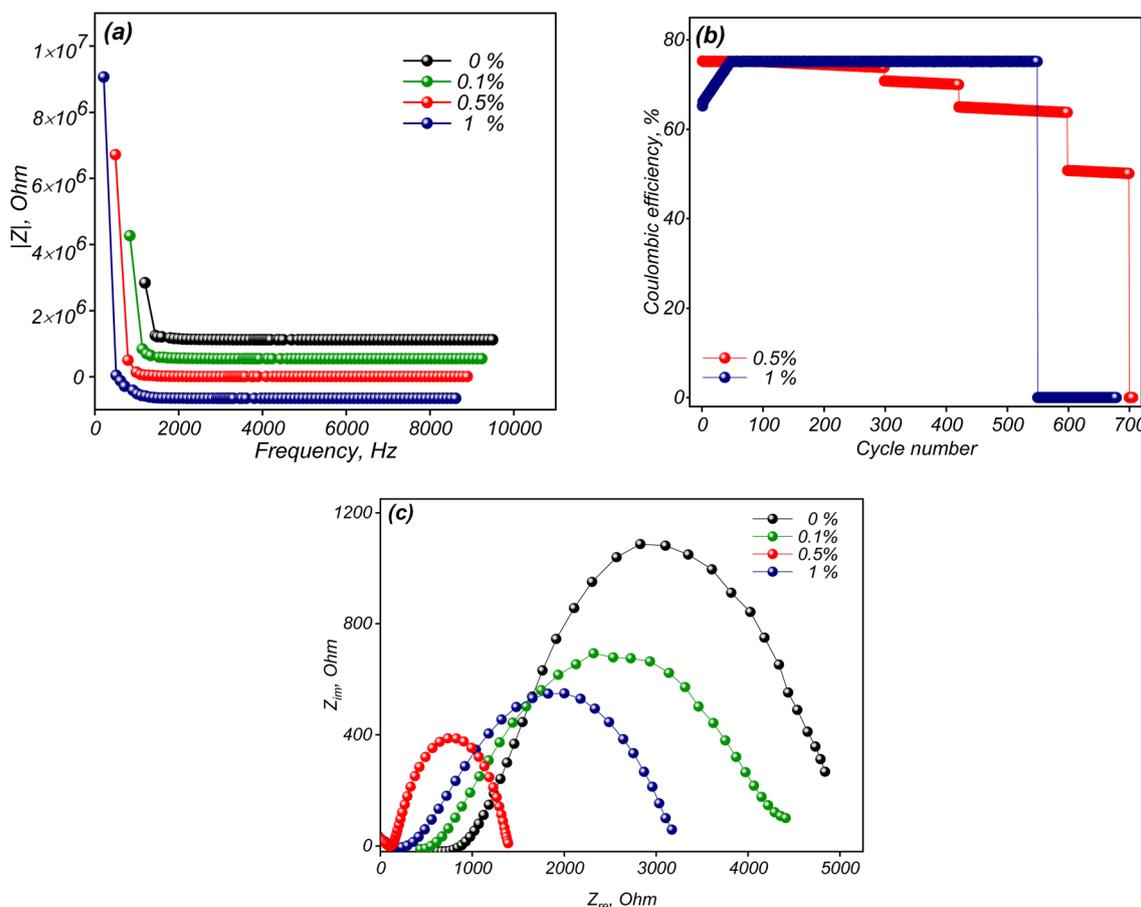
Fig. 11 Variation of the real part of impedance ( $Z'$ ) as a function of frequency for solid-state supercapacitors with different GO content (a), coulombic efficiency of supercapacitors with different GO contents (0.5% and 1%) over cycling (b), and Nyquist plot of the EIS tests (c).
