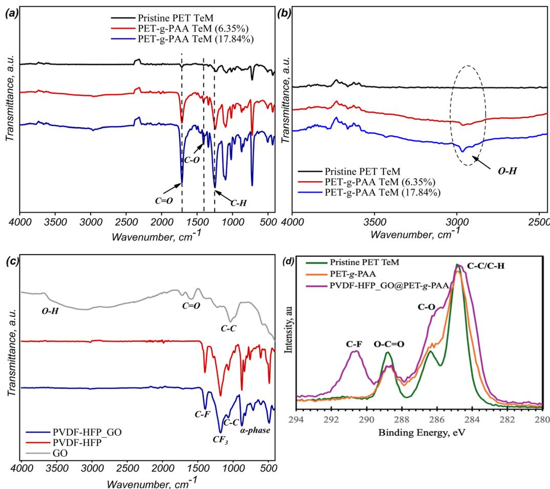
Fig. 3 FTIR spectra of PET-g-PAA in the range of  $4000\text{--}500\text{ cm}^{-1}$  (a) and  $4000\text{--}2000\text{ cm}^{-1}$  (b), FTIR spectra of PVDF-HFP\_GO nanofibers (c) and C1s core level XPS spectra of pristine PET TeM, PAA grafted membrane and PVDF-HFP\_GO@PET-g-PAA membranes (d).
