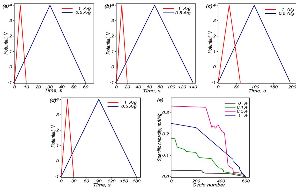
Fig. 10 Galvanostatic charge–discharge (GCD) curves of SSC with varying GO content at two different current densities of 0.5 and  $1.0 \text{ A g}^{-1}$ : 0% GO (a), 0.1% GO (b), 0.5% GO (c), 1% GO (d) and specific capacity vs. cycle number for the different compositions (e).
