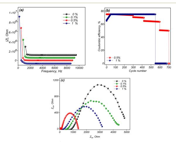
Fig. 11 Variation of the real part of impedance (Z') as a function of frequency for solid-state supercapacitors with different GO content (a), coulombic efficiency of supercapacitors with different GO contents (0.5% and 1%) over cycling (b), and Nyquist plot of the EIS tests (c).
