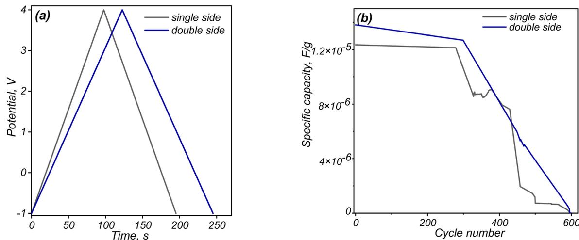
Fig. 15 GCD curves of SSC whose single-side and double-side covered with 0.5% GO containing nanofibers at a current density of  $0.5 \text{ A g}^{-1}$  (a), and specific capacity vs. cycle number for these two compositions (b).
