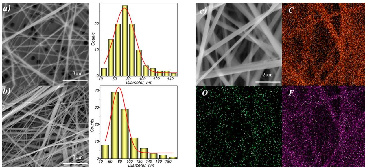
Fig. 5 SEM images of PVDF-HFP\_GO@PET-g-PAA (a) 5 min, (b) 10 min, (c) 15 min; the corresponding size distributions and elemental mappings of composite nanofibers.
