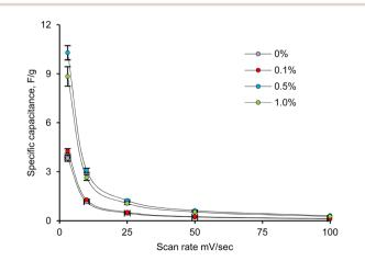
Fig. 9 Dependence of the specific capacitance on the scan rate for PVDF-HFP\_GO@PET-g-PAA with the different concentrations of GO.
