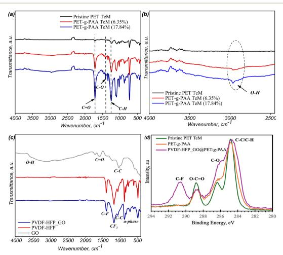
Fig. 3 FTIR spectra of PET-g-PAA in the range of 4000–500 cm<sup>-1</sup> (a) and 4000–2000 cm<sup>-1</sup> (b), FTIR spectra of PVDF-HFP\_GO nanofibers (c) and C1s core level XPS spectra of pristine PET TeM, PAA grafted membrane and PVDF-HFP\_GO@PET-g-PAA membranes (d).
