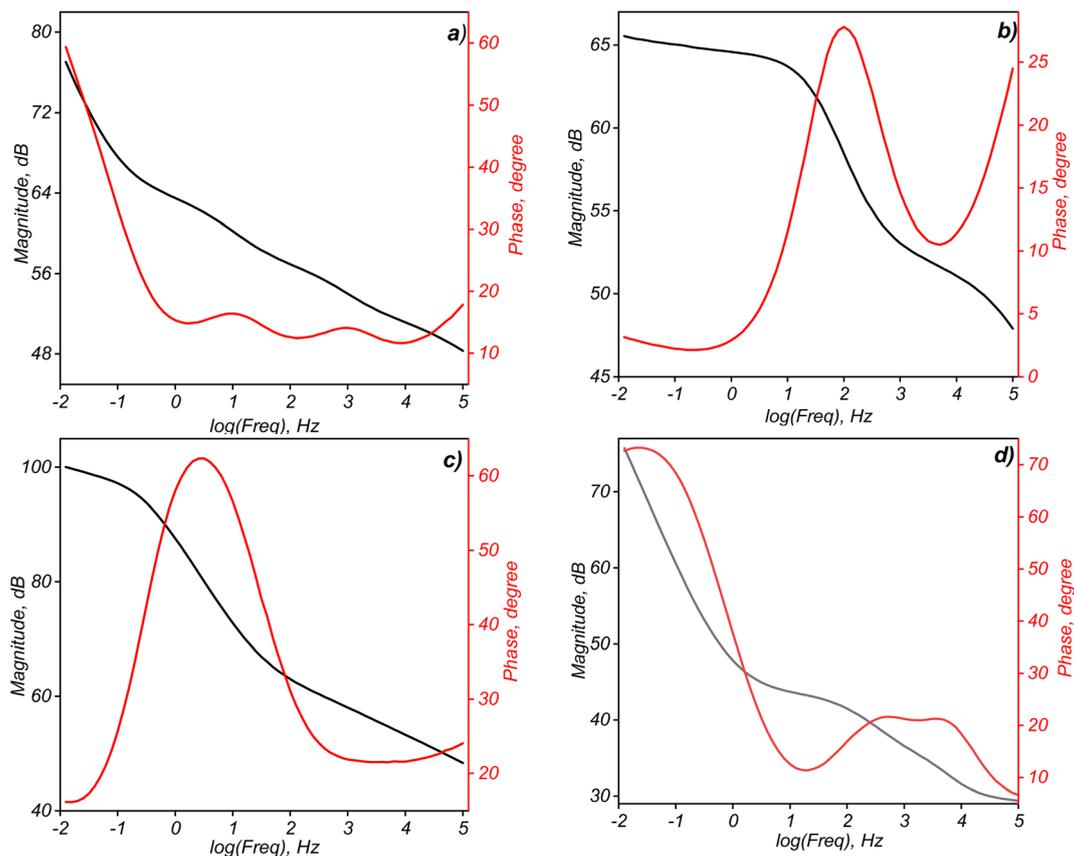
Fig. 13 Bode plot as a function of frequency for PVDF-HFP\_GO@PET-g-PAA solid-state supercapacitors with various GO content: 0% GO (a), 0.1% GO (b), 0.5% (c), 1% GO (d).
