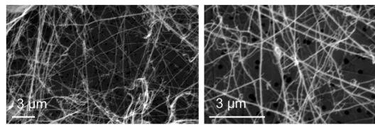
Fig. 12 SEM images of the single-side covered with 0.5% GO nanofibers GPE TeM after 600 cycles of testing at the different magnifications.
