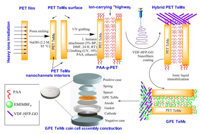
Fig. 1 General scheme of PVDF-HFP\_GO@PET-g-PAA hybrid TeM synthesis
