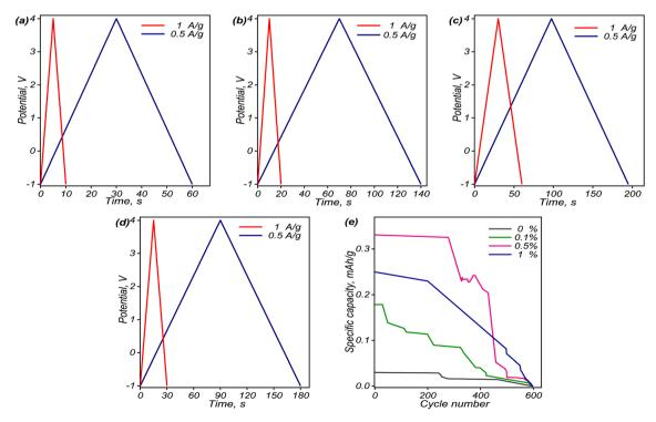
Fig. 10 Galvanostatic charge-discharge (GCD) curves of SSC with varying GO content at two different current densities of 0.5 and 1.0 A g<sup>-1</sup>: 0% GO (a), 0.1% GO (b), 0.5% GO (c), 1% GO (d) and specific capacity vs. cycle number for the different compositions (e).
