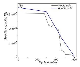
Fig. 15 GCD curves of SSC whose single-side and double-side covered with 0.5% GO containing nanofibers at a current density of 0.5 A  $g^{-1}$  (a), and specific capacity vs. cycle number for these two compositions (b).
