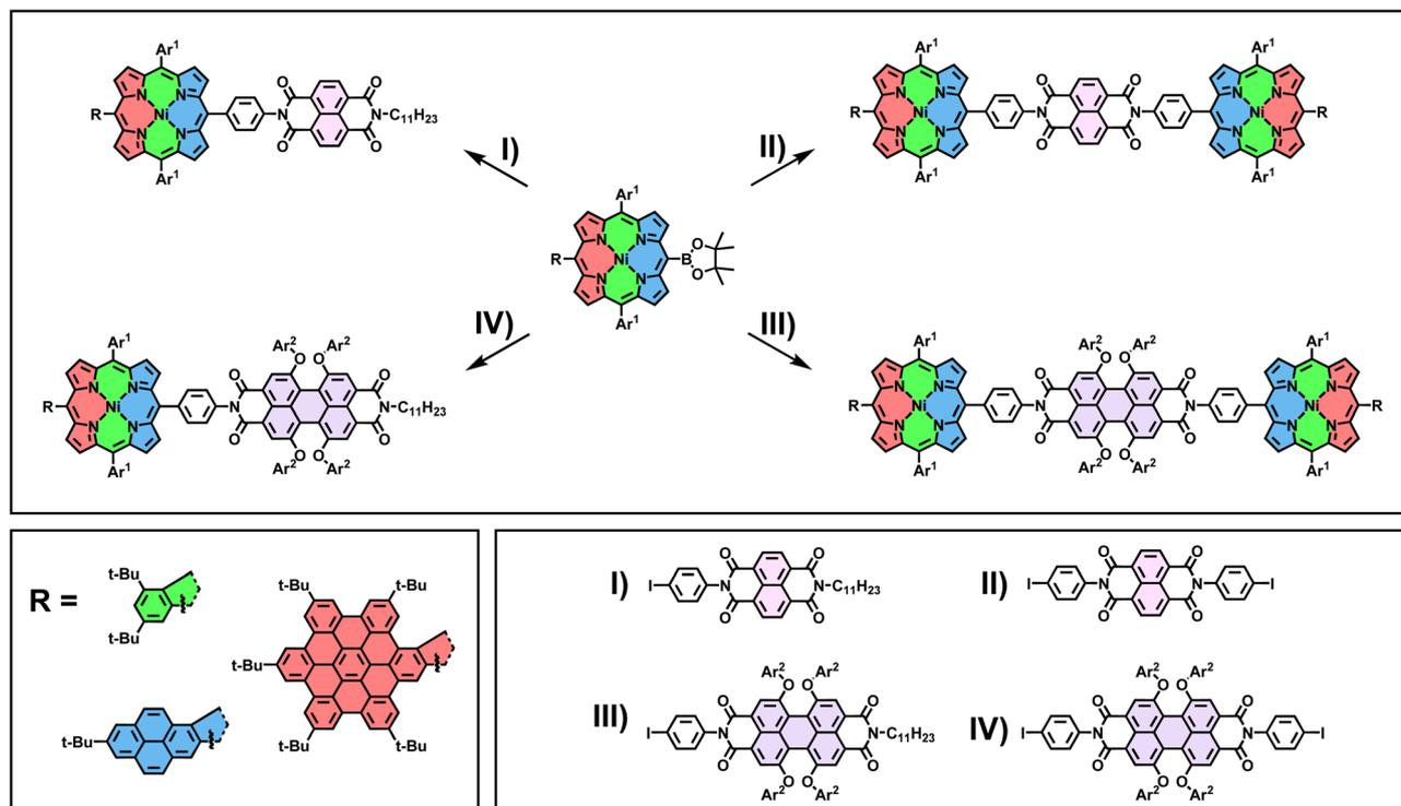
Scheme 2 Reagents and conditions: Pd(PPh<sub>3</sub>)<sub>4</sub>, Cs<sub>2</sub>CO<sub>3</sub>, toluene/DMF 2 : 1, 18 h, 80 °C. Ar<sup>1</sup> = mesityl; Ar<sup>2</sup> = 4-*tert*-butylphenyl.
