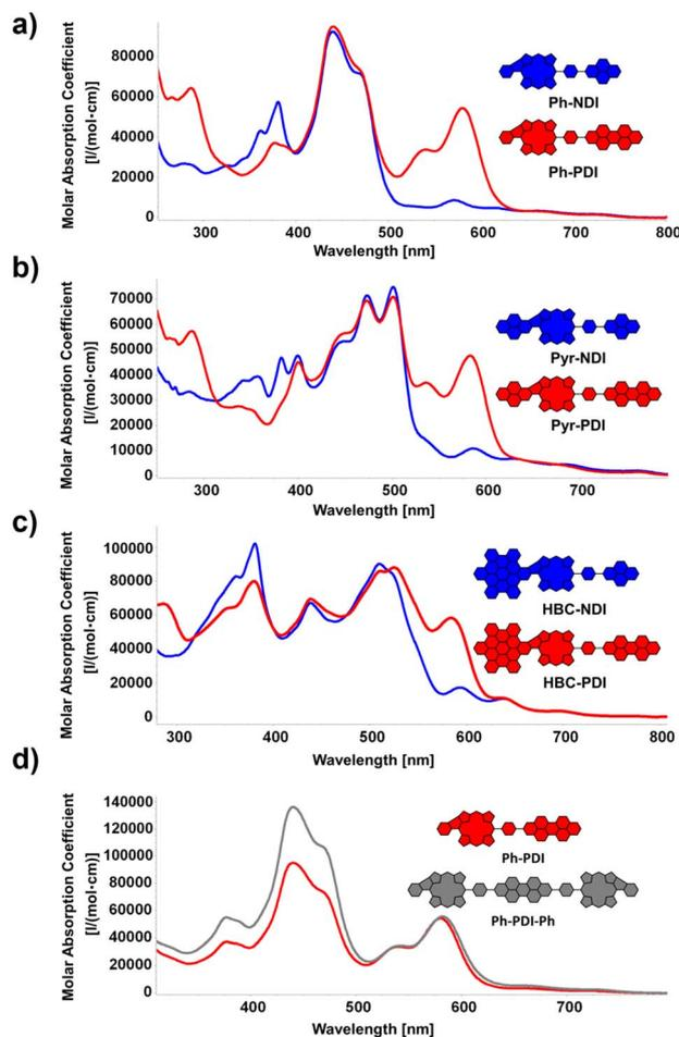
Fig. 4 (a)–(c) UV/vis spectra of the D–A dyads. Solvent:  $\text{CH}_2\text{Cl}_2$ . (d) Comparison of UV/vis spectra of dyad Ph-PDI and respective triad Ph-PDI-Ph. Solvent:  $\text{CH}_2\text{Cl}_2$ .
