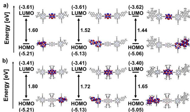
Fig. 6 Eigenvalues and orbital contours of the HOMO and LUMO of (a) the NDI-based triads Ph-NDI-Ph, Pyr-NDI-Pyr, and HBC-NDI-HBC (left to right); (b) the PDI-based triads Ph-PDI-Ph, Pyr-PDI-Pyr, and HBC-PDI-HBC (left to right) in the gas phase calculated at DFT (B3LYP/def2-TZVPP) level of theory including an implicit solvation model.
