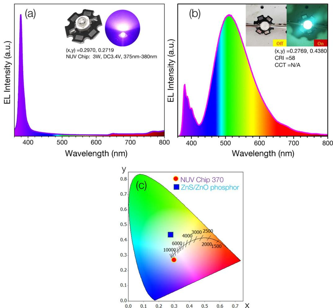
Fig. 7 (a) EL spectrum of NUV chip (370 nm, 3 W, 3.4 V); (b) EL spectra of NUV-pumped ZnS/ZnO phosphor; (c) the CIE 1931 chromaticity diagram of the fabricated cyan-LED and NUV-chip.
