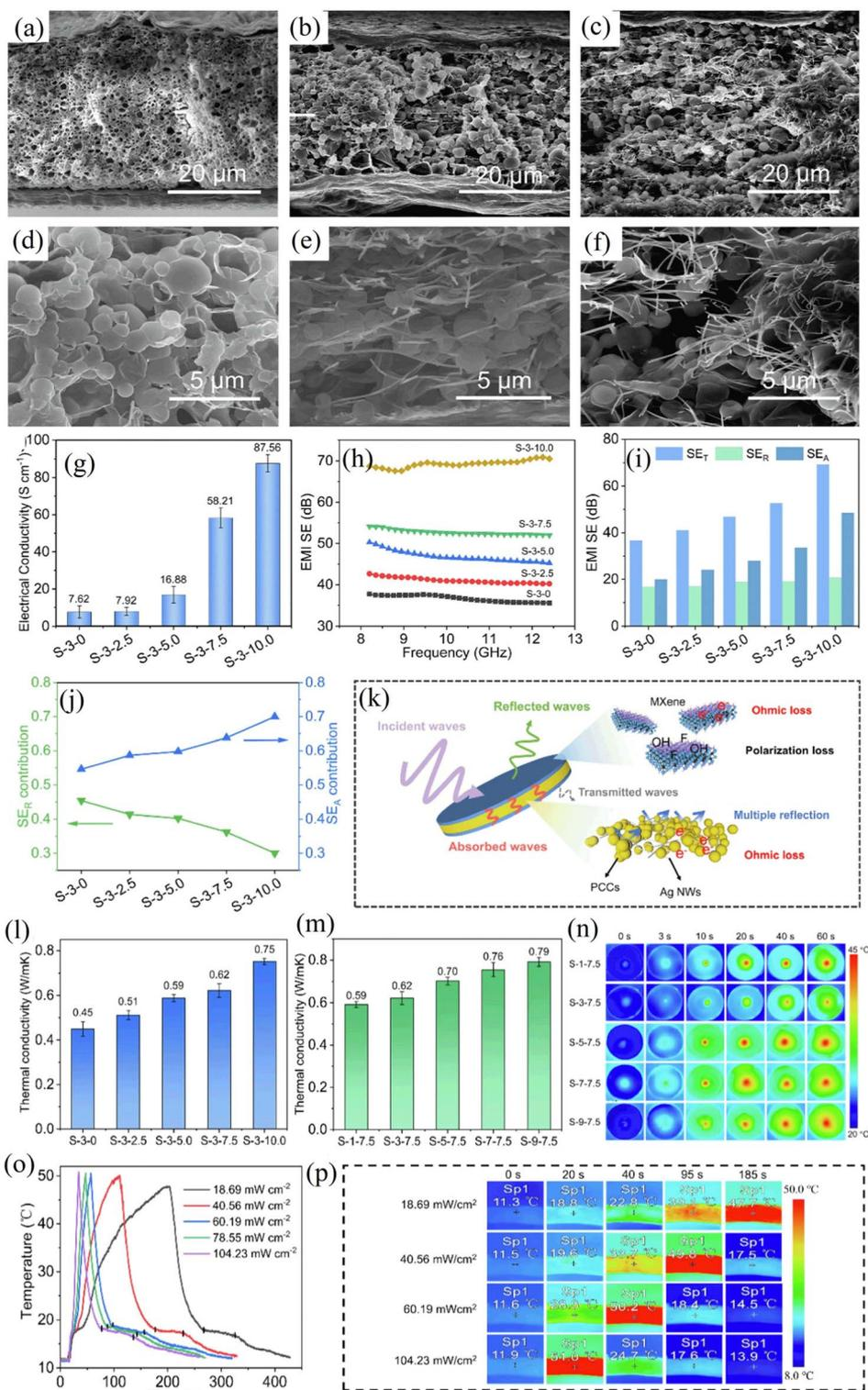
Fig. 7 (a–f) Scanning electron microscopy (SEM) schematic of sandwich composite films, (g–j) characterization of conductivity and electromagnetic shielding properties of sandwich composite films, (k) electromagnetic shielding mechanism diagram of sandwich composite films, (l–p) photothermal characterization of sandwich composite films. Reproduced from ref. 112 with permission from [Elsevier], copyright [2024].
