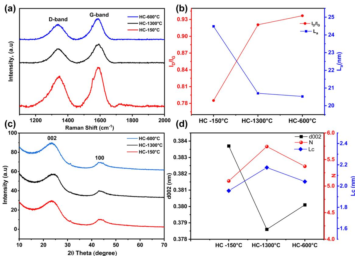
Fig. 3 (a and b) Raman spectrum data; (c and d) XRD data and  $d_{002}$  spacing and stacking thickness.
